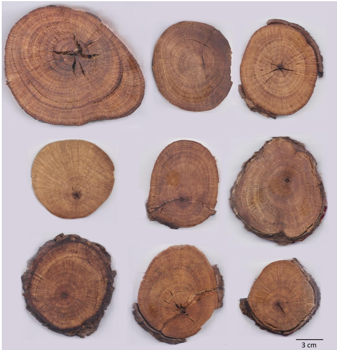
Figure 2. The polished witness disks. Top row: S1-S3, middle row: S4-S6, bottom row: S8-S10. The witness for S7 cracked radially from the pith outward and handling was kept to a minimum; it is not included in this image. 'S' is used to denote stem.
