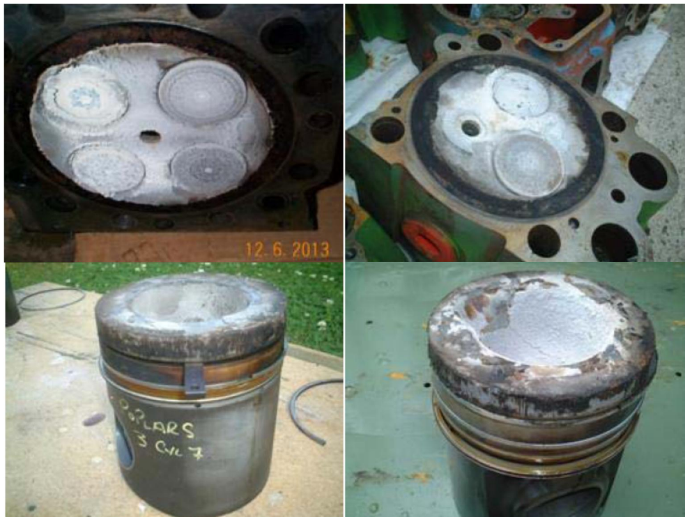
Figure 2.10: Silica build up on heads and scrapped pistons of Caterpillar and Jenbacher engines (Xebec Adsorption Inc., 2007)
