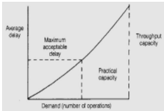
Figure 2-2: Relationship between throughput and practical capacity. Wells (2000:244)
