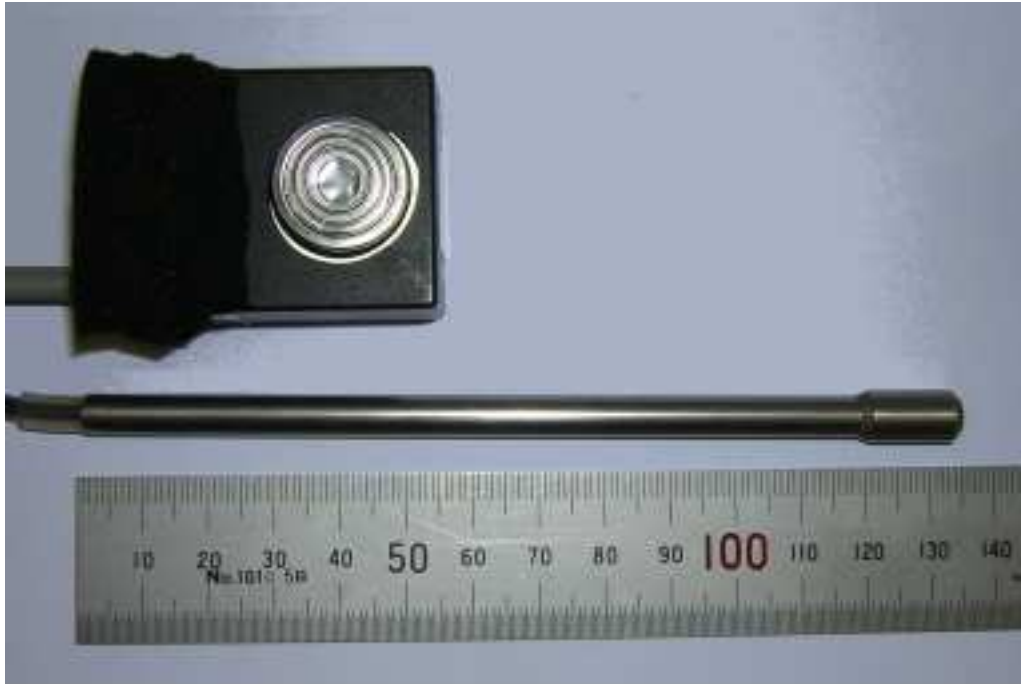
Figure 3.3: Comparison of different sensors. The top sensor is the IC-Sensor enclosed in a plastic housing and the bottom sensor is the hand held probe from Millar Instruments, which is used in the Sphygmocor system.
