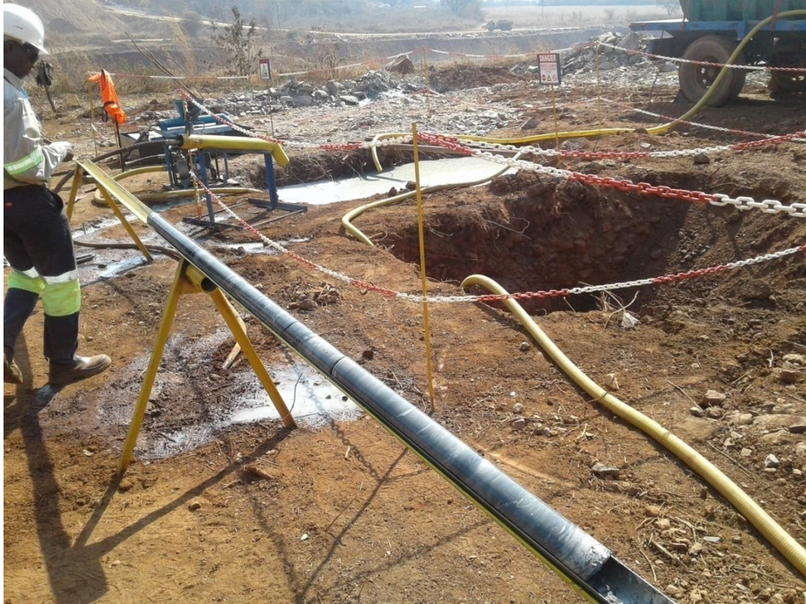
Figure 3-8 Drilled core just after removal from the core barrel and cleaned, lying on the angle iron core stand (Courtesy of Pickstone-Peerless Mine).
