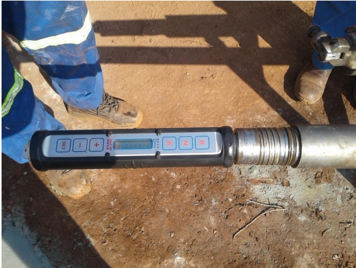
Figure 3-6 Determining the in situ core orientation with a Reflex ACT III orientation tool connected to the upper end of the core barrel whilst the core is inside the core barrel (Courtesy of Pickstone-Peerless Mine).
