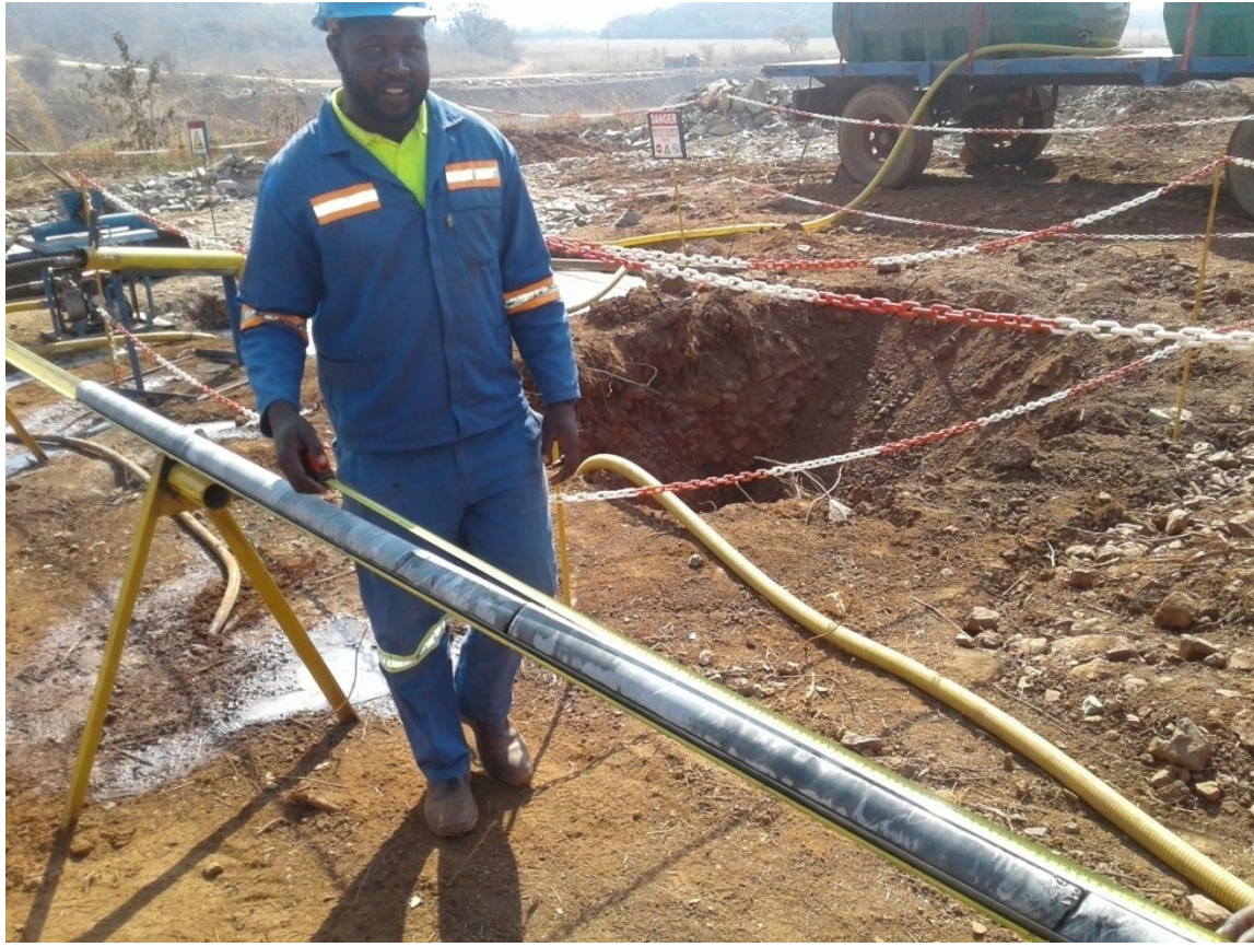
Figure 3-10 Measuring the Total Core Recovery (TRC) for a particular drill run using a steel measuring tape (Courtesy of Pickstone-Peerless Mine).
