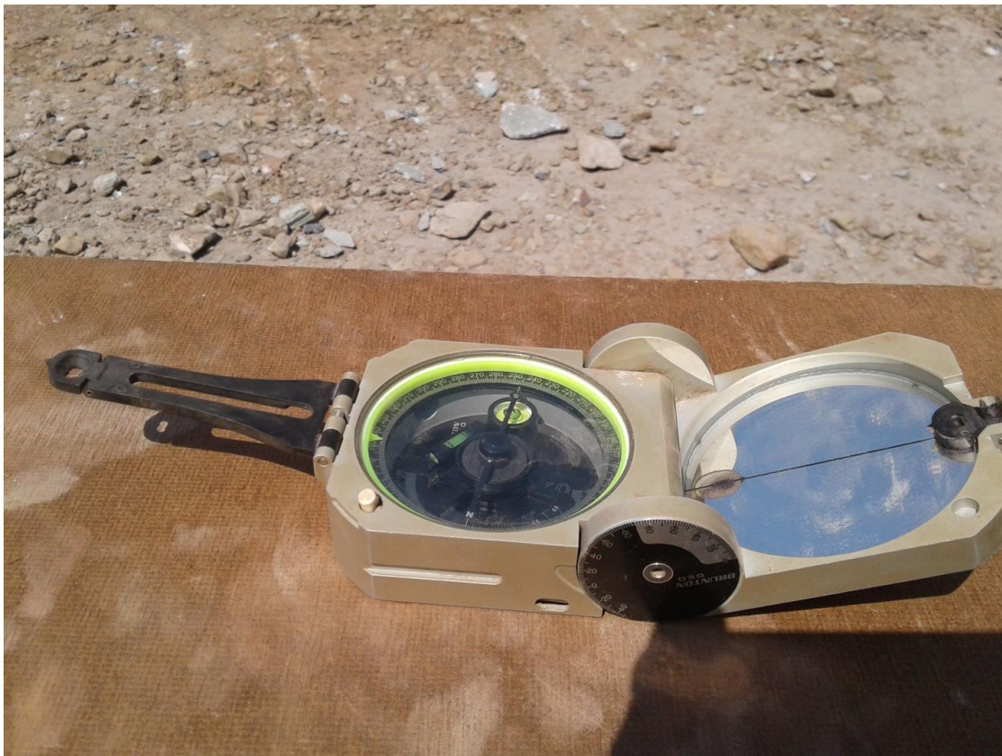
Figure 3-13 Brunton geological compass that was used to measure dip and dip direction during face mapping.
