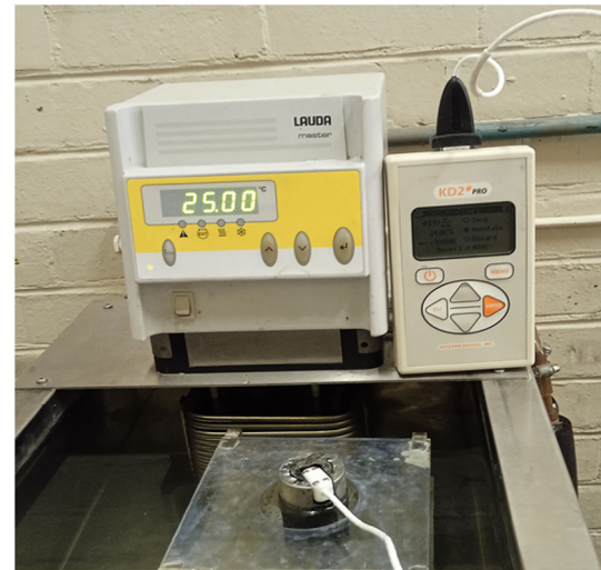
Fig. 3 Experimental setup for thermal conductivity measurement
