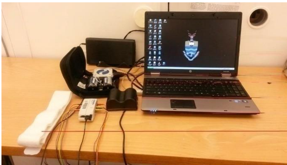
Figure 2.7. Showing the Cadwell Easy Ambulatory system set up. The Cadwell Easy Ambulatory system consisted of a D-cell battery powered recorder and amplifier (image taken from the Wits sleep laboratory, polysomnography standard operating system).
