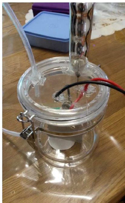
Figure A2: Experimental set-up with mechanical agitator for activity determination investigation
