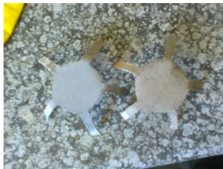
Figure 42: Nickel star shaped electrodes as observed after a beaker test at 2.5VDC for a testing duration exceeding 24 hours.
