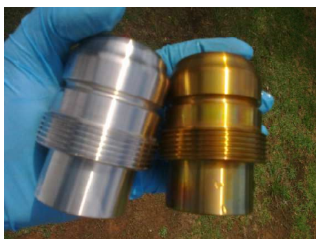
Figure 33: Left: - General silver sheen of the cathodic conductive head. Right: - Altered appearance to a bronze appearance of the anodic conductive head.
