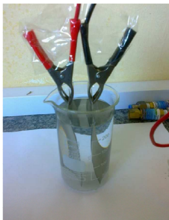
Figure 40: Bench top experimental set-up configuration for the determination of a suitable stable conductive material
