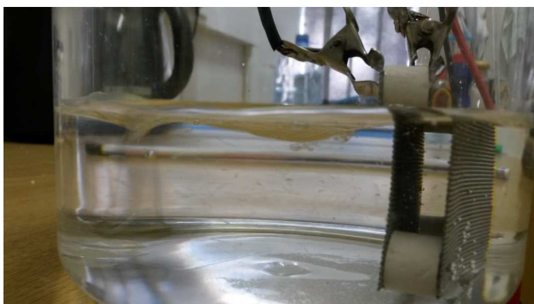
Figure A3: Agitation system in motion moving fluid over the porous mesh electrodes
