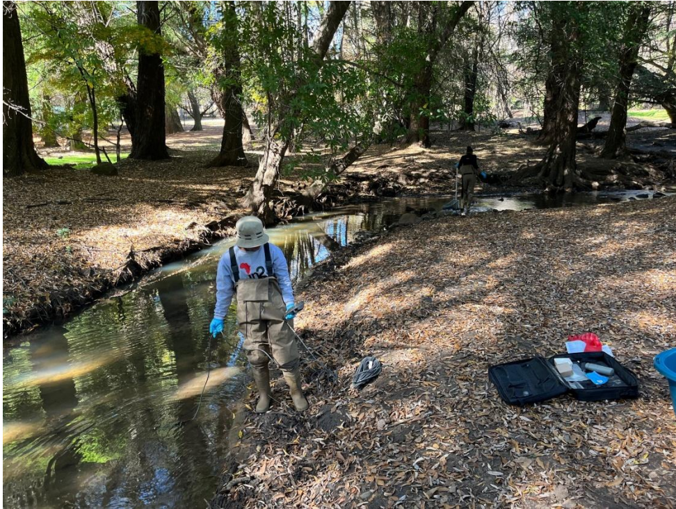
Figure 8: The waders used to take samples and the YSI used to take in-situ measurements
