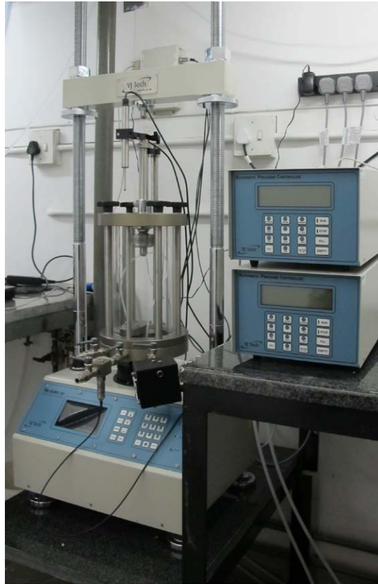
Figure 7.16 Triaxial testing Setup 1: automated system.
