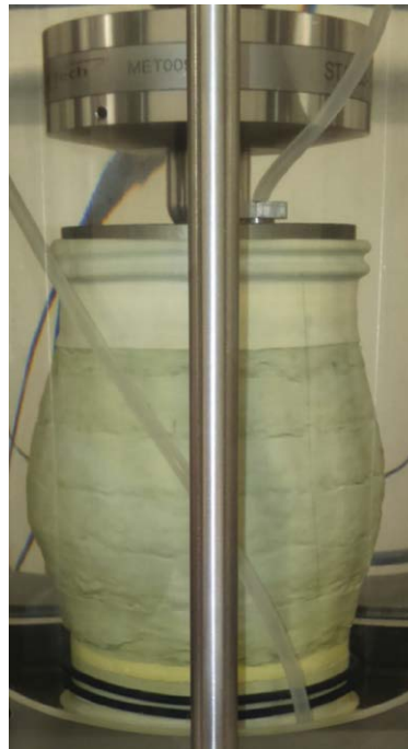
Figure 7.24 Typical barrel-like geometry of sheared specimens.
