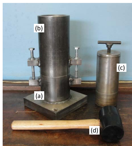
Figure 7.7 Equipment used to conduct nonstandard e_{min} determinations: a) compaction mould, b) extension sleeve, c) overburden weight, and d) rubber mallet.
