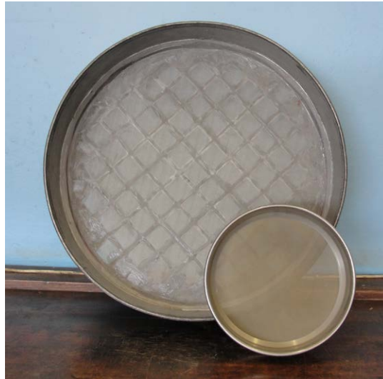
Figure 7.1 Nonstandard (450 mm diameter) and standard (200 mm diameter) sieves.
