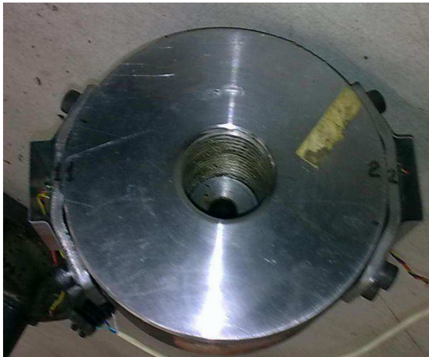
Figure 5.3: Positioning and casing for the accelerometer circuits.
