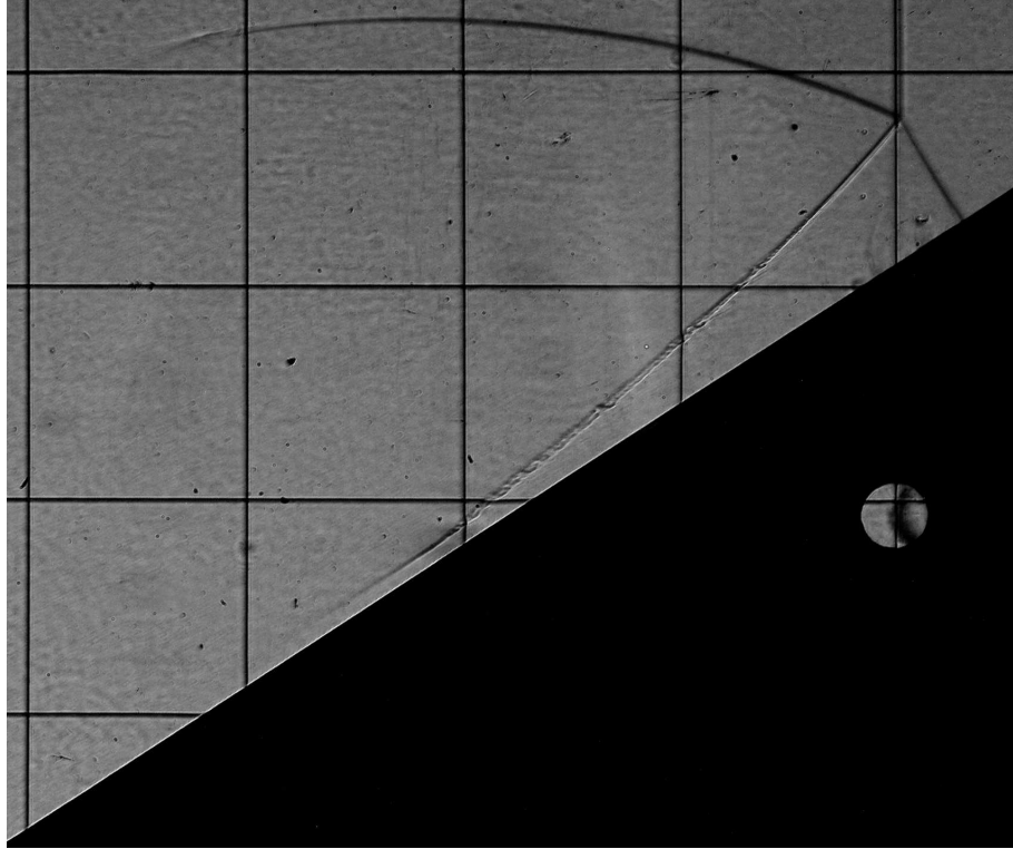
Figure 8.1: Schlieren image, with camera-side knife edge perpendicular to the shear layer, of flow field progression for Model D ( M_0 = 1.46 ).
