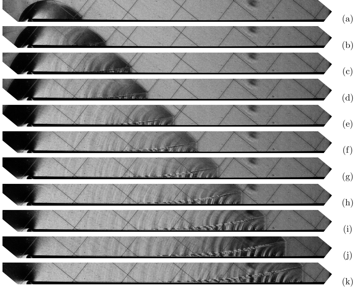
Figure C.18: KHI evolution for Model F, M_0 = 1.61 . At times of (a) 1440\mu s , (b) 1460\mu s , (c) 1480\mu s , (d) 1500\mu s , (e) 1520\mu s , (f) 1540\mu s , (g) 1560\mu s , (h) 1580\mu s , (i) 1600\mu s , (j) 1620\mu s and (k) 1640\mu s .
