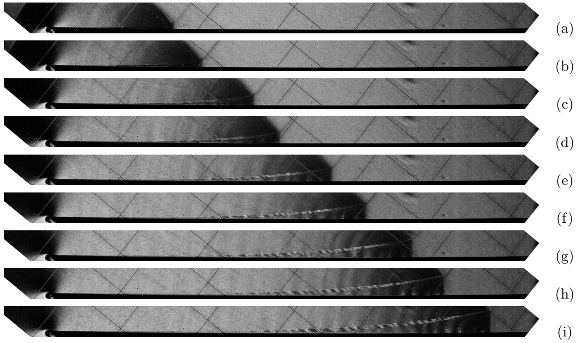
Figure C.17: KHI evolution for Model F, M_0 = 1.46 . At times of (a) 1600\mu s , (b) 1625\mu s , (c) 1650\mu s , (d) 1675\mu s , (e) 1700\mu s , (f) 1725\mu s , (g) 1750\mu s , (h) 1775\mu s , and (i) 1800\mu s .
