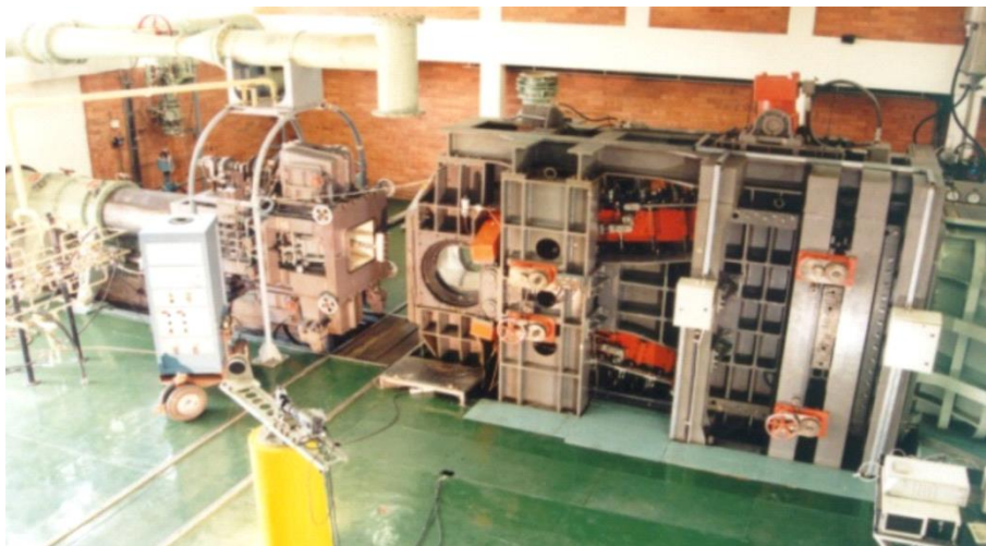
Figure 1.1: CSIR's supersonic wind tunnel facility (HSWT)
