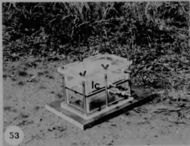
Fig.52 Shimshi apparatus for measuring gross photosynthesis. C- 14 CO 2 gas cylinder, CL - clamp, arrow - leaf chamber. Fig.53 Cuvette for holding leaf specimens. Wj - water jacket, lc - leaf chamber, solid arrows - air inlet, open arrows - water inlet.
