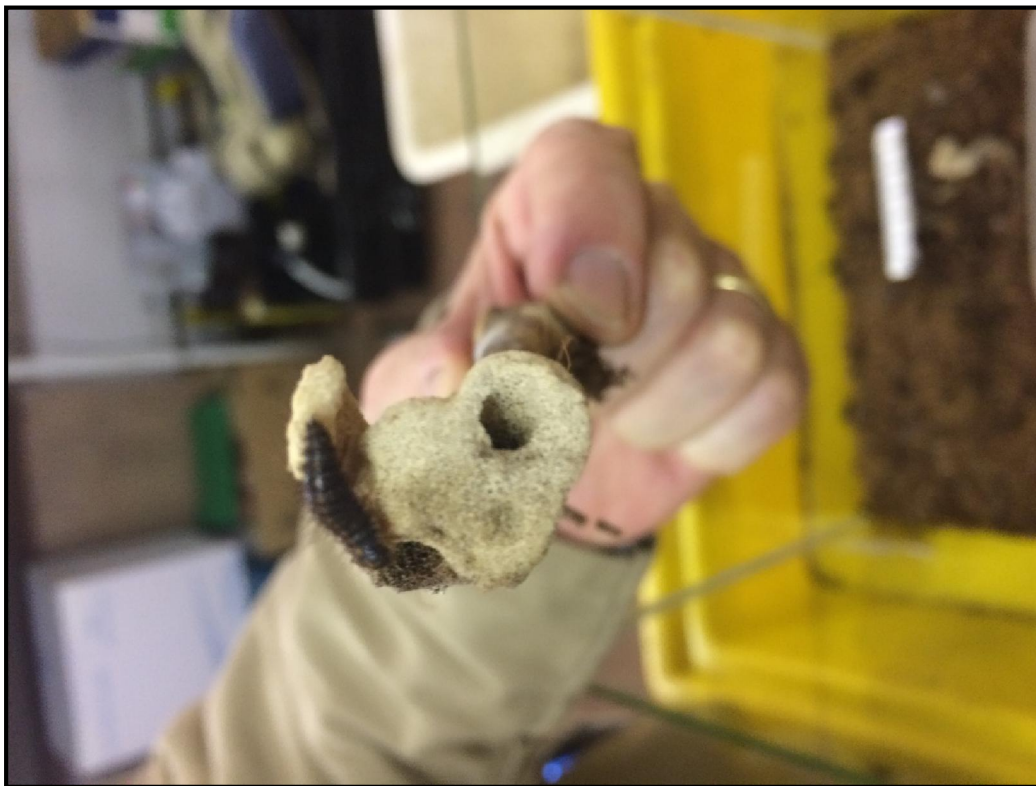
Figure 13. Macro view of bore hole damage on chicken raw ii.
