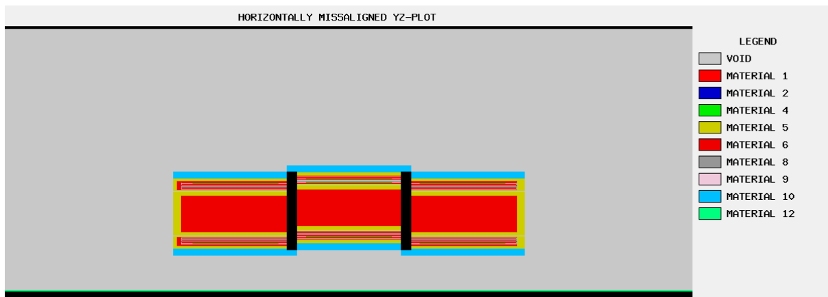
Figure 4.14: 3 X 10 storage array in a horizontal orientation with the middle row elevated by 20 cm.
