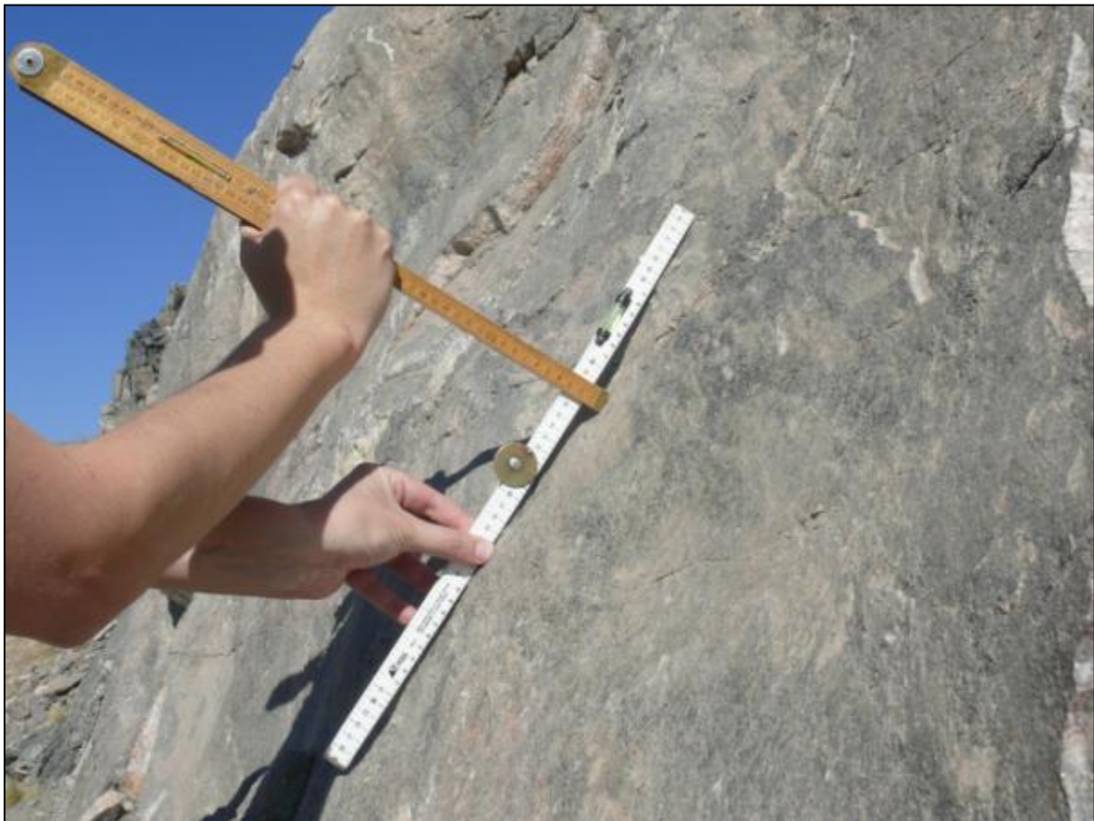
Figure 6.4 Illustrating how the roughness or unevenness amplitudes were measured on a 500mm scale.
