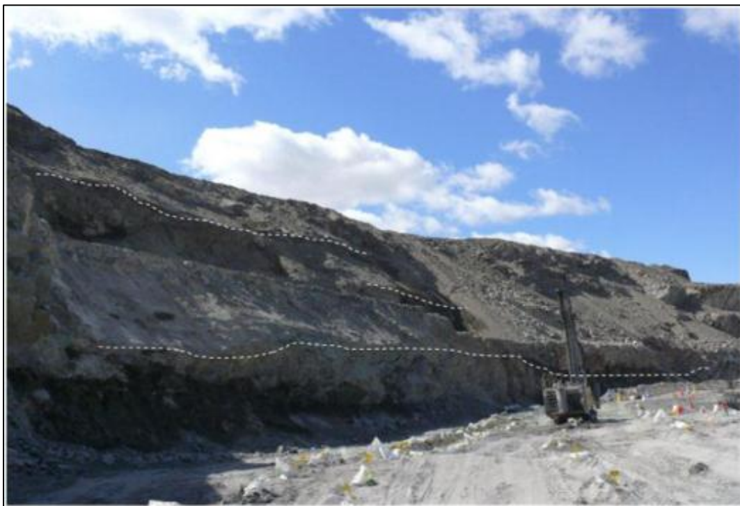
Figure 1.14 MS3 structure in the East-wall of Cut 4 with the typical infilling. S2 is striking perpendicular to the wall.
