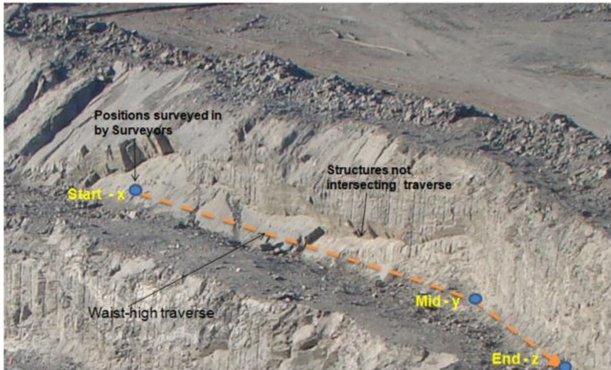
Figure 5.1 Diagram representing a scan line and showing the waist high imaginary traverse.
