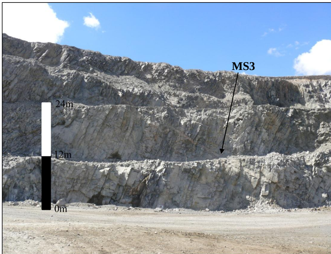
Figure 1.14 MS3 structure in the East-wall of Cut 4 with the typical infilling. S2 is striking perpendicular to the wall.
