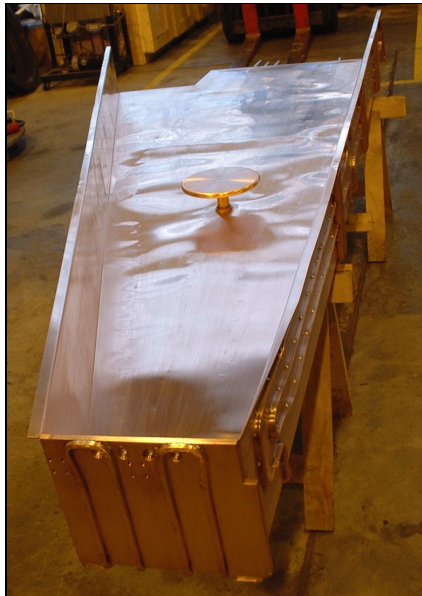
Figure 6.13. The capacitor connected to the outer conductor of the resonator. It is used for coarse tuning and electro-magnetic balancing of the upper and lower halves of the resonator.
