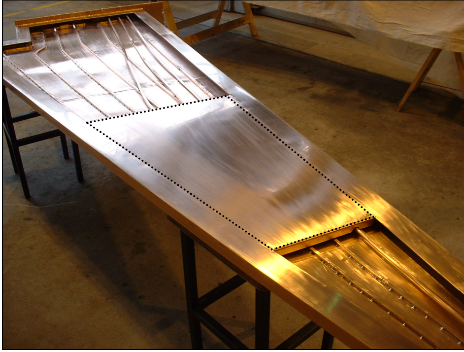
Figure 5.22. A copper plate welded to the inside of a dee plate (indicated with a dotted line) for separation of the two resonance frequencies. The addition of the plate decreased the resonance frequency of the unwanted mode by about 6 MHz without affecting the frequency of the wanted mode.
