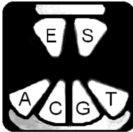
Figure 2.7: PyromarkMD Cartridge. Arrangement of tips in the Pyrosequencing MD Cartridge. S - Substrate; E- Enzyme; A,C,G,T- 4 nucleotides.
