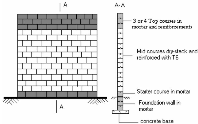
Figure 7.5 Wall cross-section details
