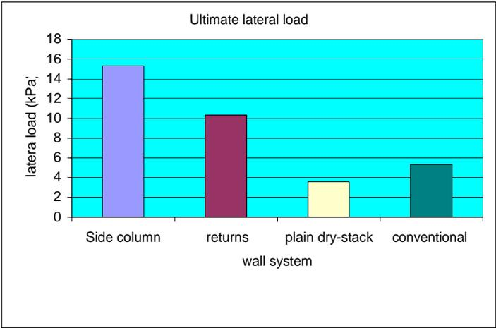
Figure 7.10 Load capacity of wall systems
