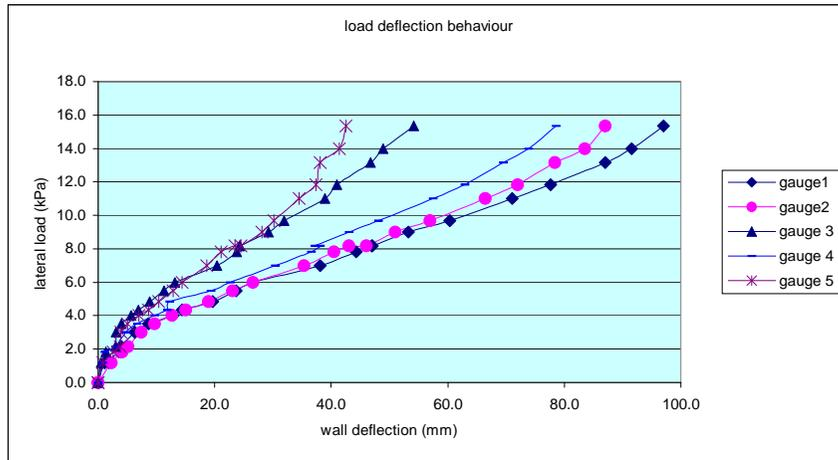
Figure 7.7 Load - deflection behaviour under lateral load.
