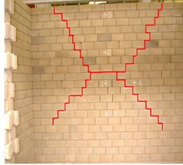
a) casting side columns in steel forms                      b) mode of failure
