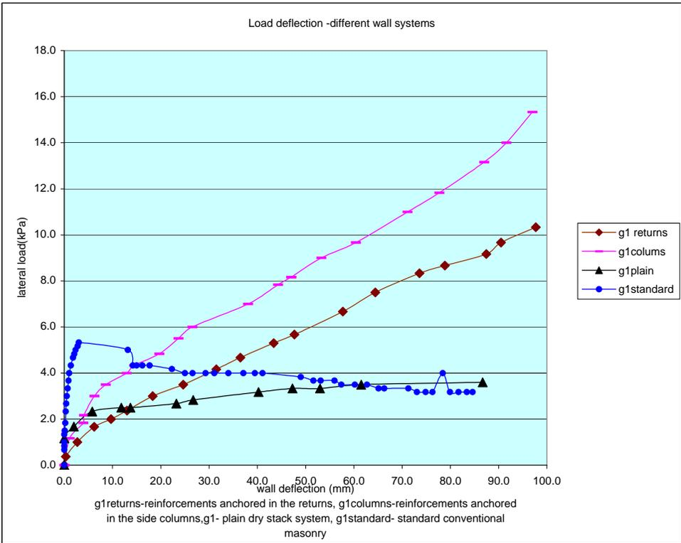
Figure 7.9 Load-deflection – different wall systems
