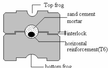
(b) placements of horizontal reinforcement
