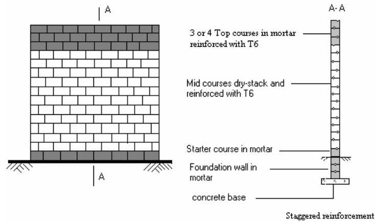
Figure 7.8 Wall cross-section – seismic block type II
