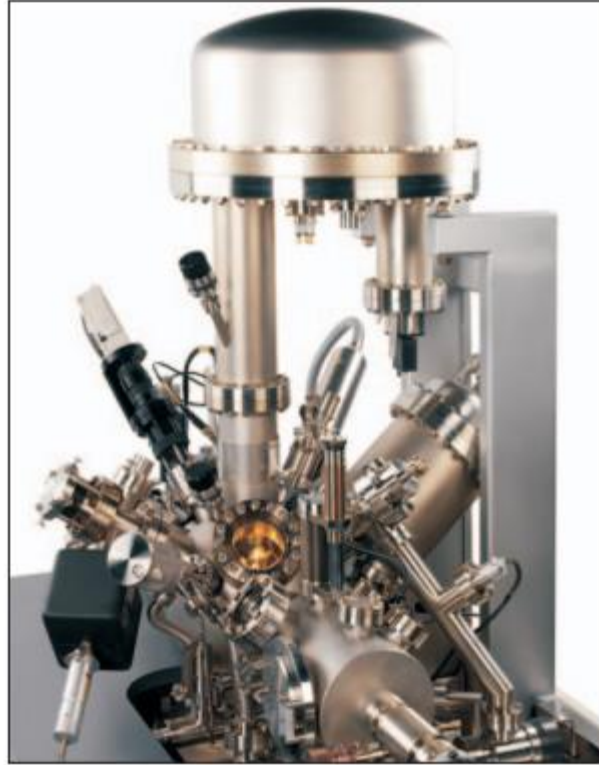
Figure 3.8: Picture of the Thermo ESCALab 250Xi X-Ray Monochromatic Al K \alpha (1486.7 eV).
