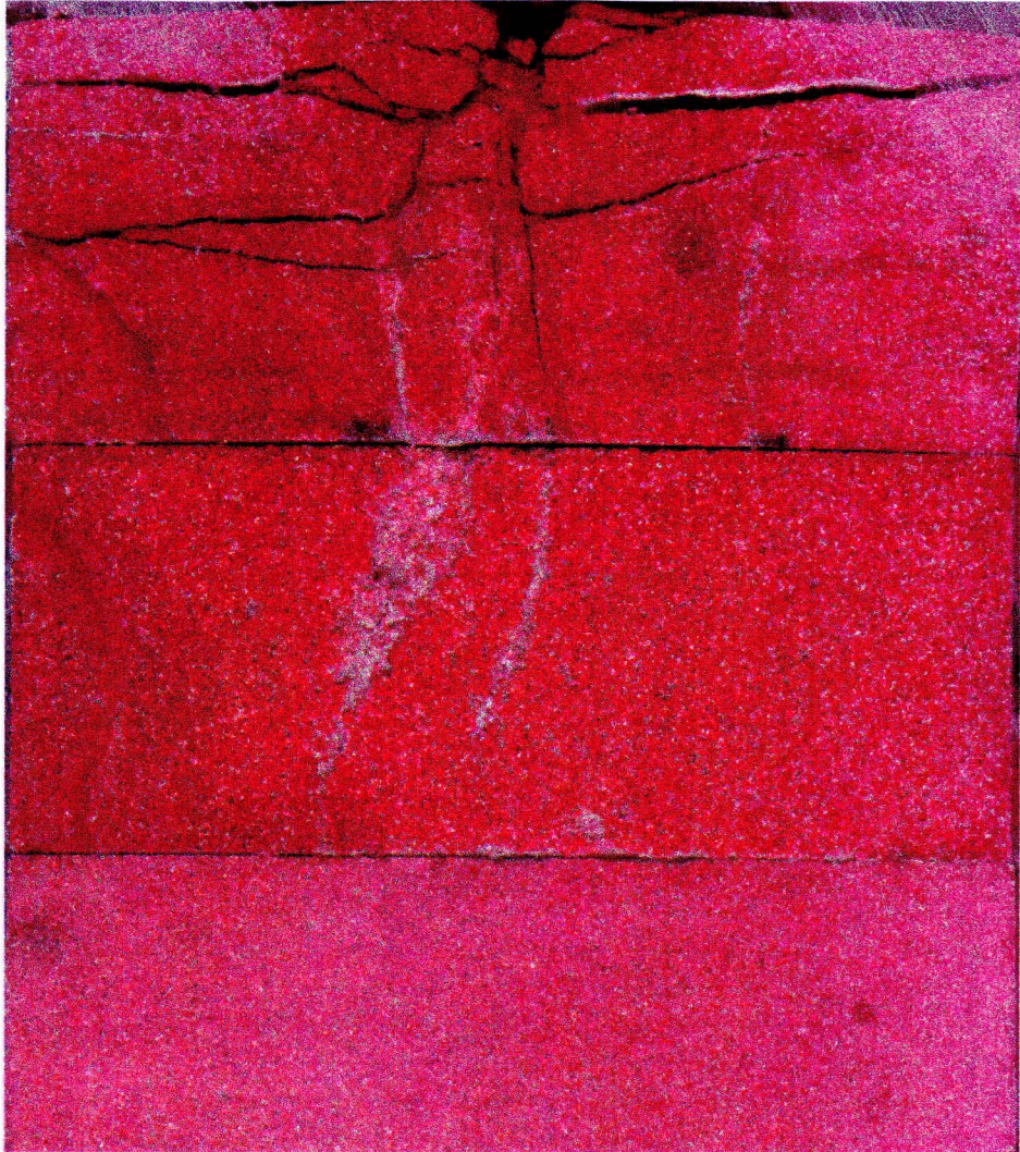
Figure D.8 20 mm layered sandstone sample from steel punch test (with friction reducer between the layers)
