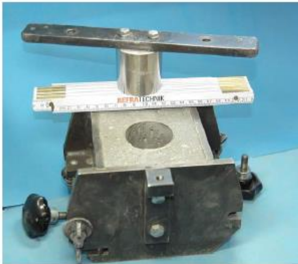
Figure 2.21: Cup/Pot static test for slag-metal corrosion test method (Kesseheim 2008)
