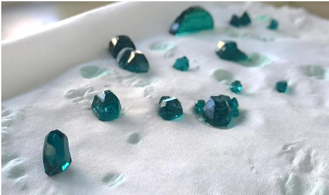
Figure 2.1: Solid nickel (II) sulphate hexahydrate \text{NiSO}_4 \cdot 6\text{H}_2\text{O} crystals (Mabowa et al., 2024)
