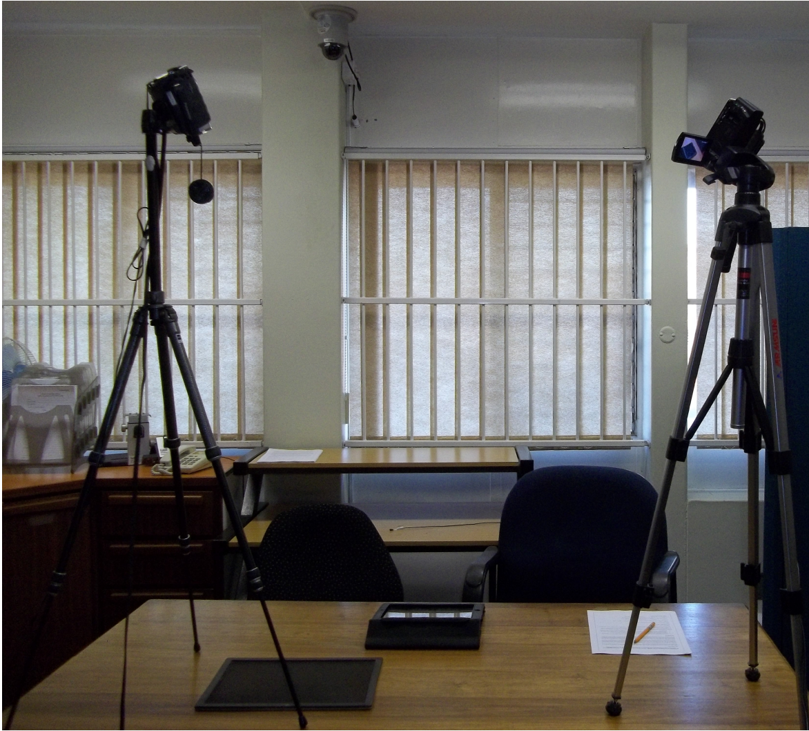
Figure 1: Laboratory set-up – Standalone cameras and rear built-in camera (front built-in camera out of view)
