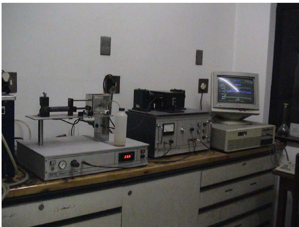
Figure 2.1 Stopped-flow spectrometer used to collect all the kinetic data in this work.
