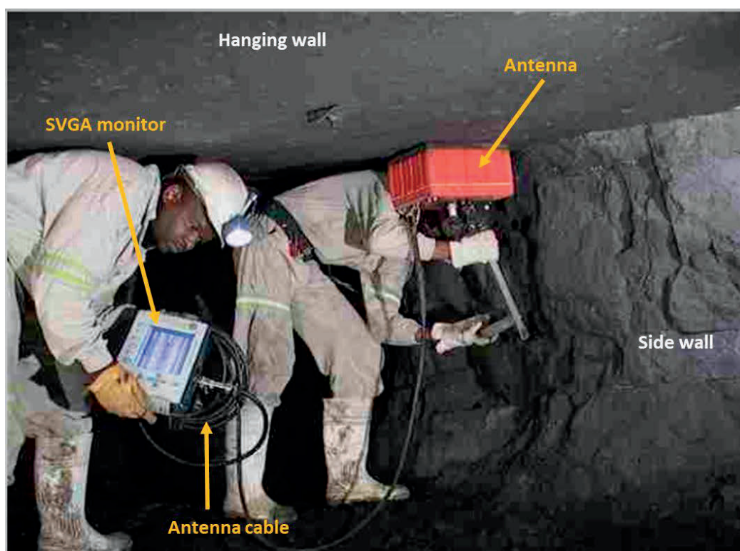
Figure 3.3: GPR scanning ( Internal Mine Document (b), 2016 )
