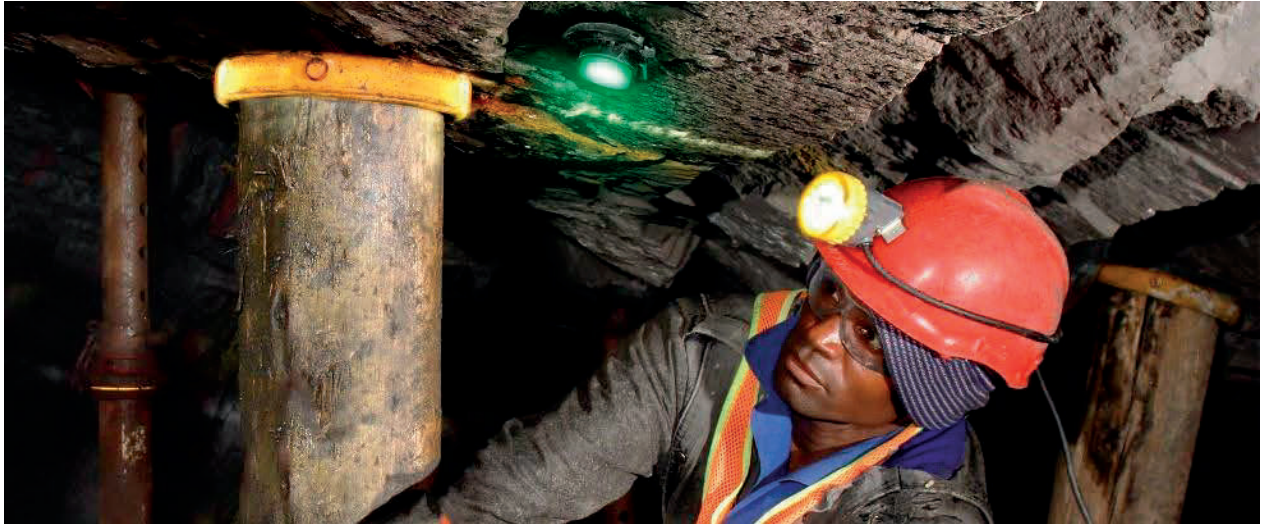
Figure 3.10: FOG light in monitoring condition (Anon, nd)
