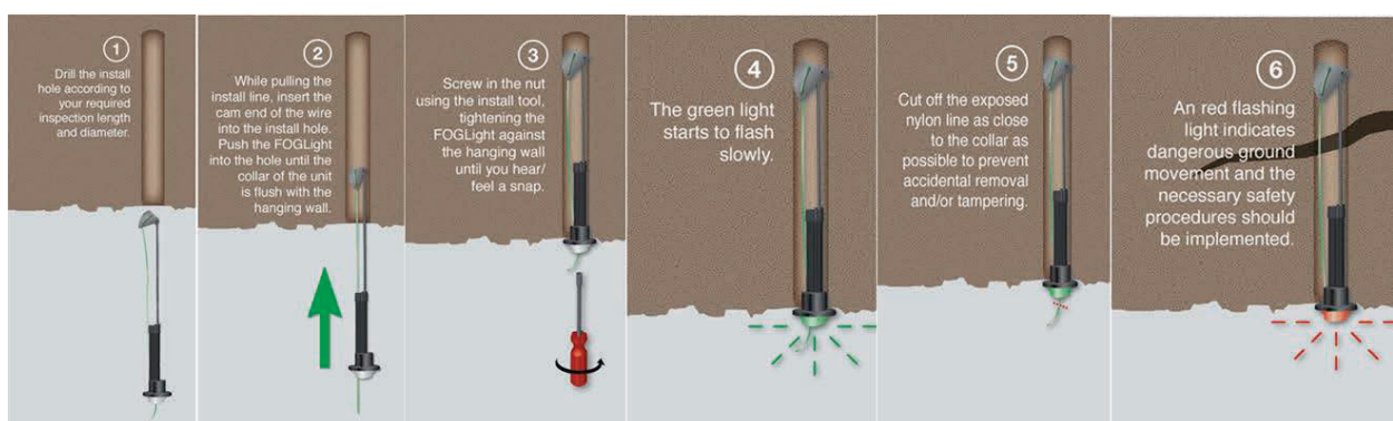
Figure 3.9: FOG light installation procedure (Anon, nd)
