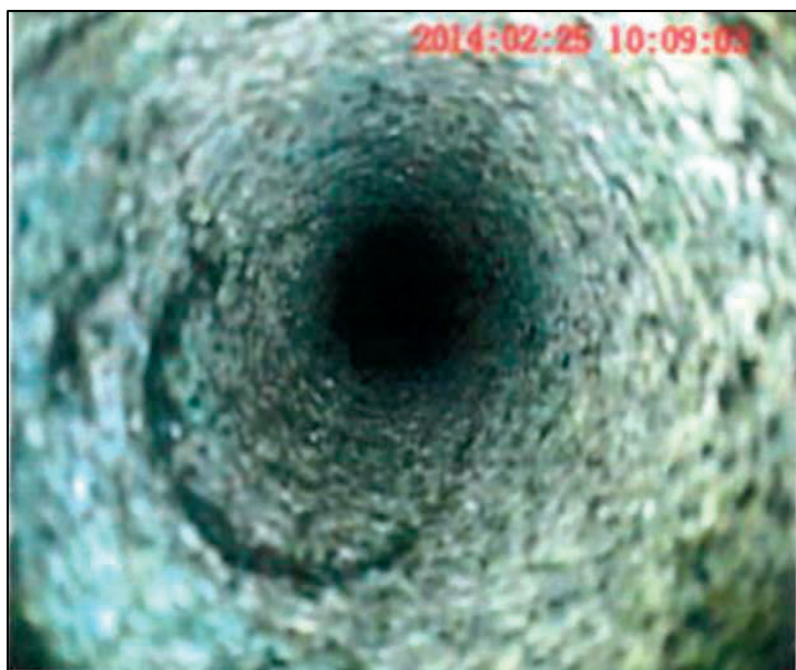
Figure 3.7: Near vertical joint observed at 2.2m in the hanging wall ( Internal Mine Document (a), 2014 )
