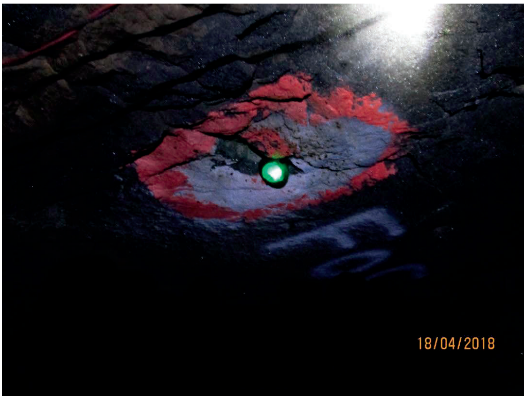
Figure 3.11: FOG light in monitoring condition at the Chrome mine
