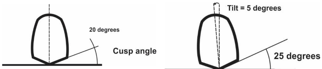
Fig. 7. The tooth on the left, upright on a flat plane, as a cusp angle of 20°. On the right, it has been tilted 5° and so the distal incline has now become 25°.
