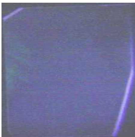
Figure 3.19: In type IIa natural diamond, the purple-blue luminescence might result from different excited states of boron acceptors in bulk or the combination of luminescence emitted by boron acceptors and the luminescence emitted by the dangling bond.
