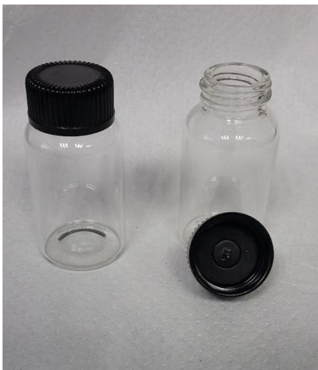
Figure 3.1: (a) The glass screw-top rubber-lined dram vials used for refluxing. The vials have a rubberized seal and can boil without significant loss of solvent. (b) When refluxing in the closed vial, solvent evaporates and flows back down the side of the vial.
