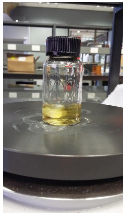
Figure 3.1: (a) The glass screw-top rubber-lined dram vials used for refluxing. The vials have a rubberized seal and can boil without significant loss of solvent. (b) When refluxing in the closed vial, solvent evaporates and flows back down the side of the vial.
