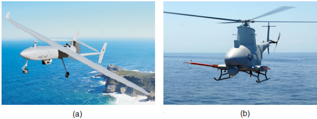
Figure 1.1: Comparing a fixed-wing (a)(Denel-Dynamics, 2018) to a single rotor rotary-wing (b)(MilitaryFactory, 2008) UAVs.
