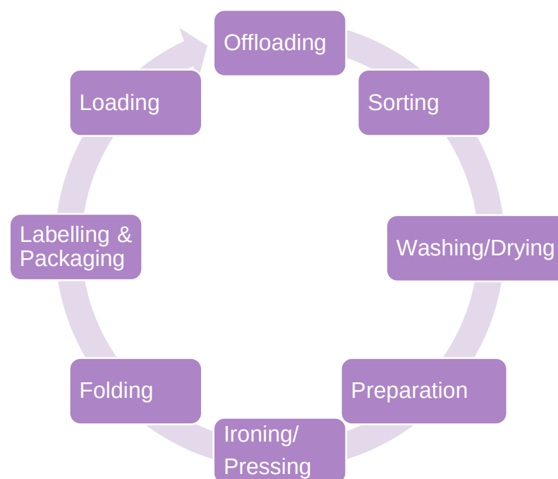
Figure 2.1: Process Flow of the Hospital Laundry
