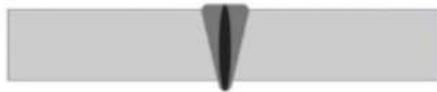
Figure 2-20: Burn through defect (Baughurst, 2011).
