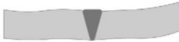
Figure 2-19: warping defect (Baughurst, 2011).
