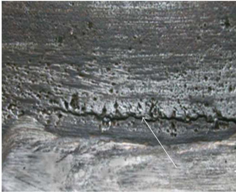
Figure 2-26: Mode 1 pitting corrosion and intergranular cracking (Amuda, 2011).
