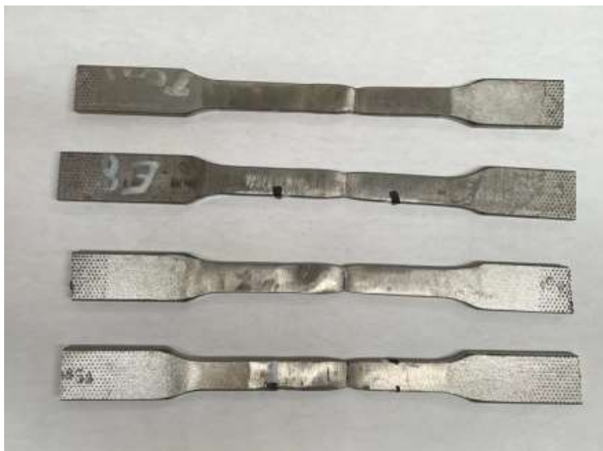
Figure 4-15: Fracture points for the tensile samples.
