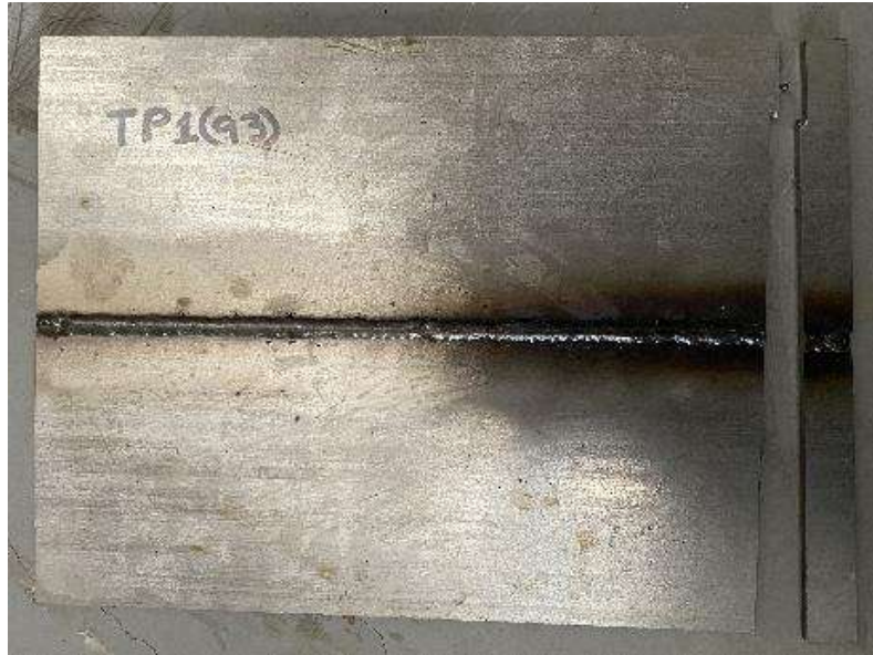
Figure 2: welded 3Cr12 plate with 308L welding wire.
