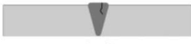
Figure 2-16: Crack defect (Baughurst, 2011).
