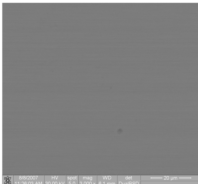
Figure 4.109. BSE-SEM image of nominal 64 at.% Pt annealed at 1400°C, showing Pt 3 Al single phase.
