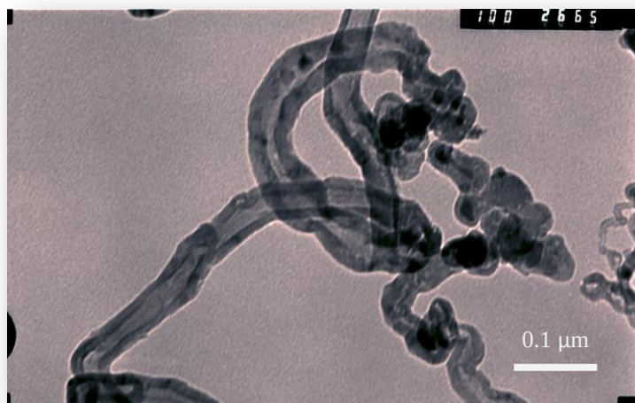
Figure 4.2: Typical TEM micrograph of MWCNTs after 1:3 HNO 3 :H 2 SO 4 acid treatment
