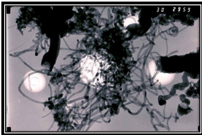
Figure A6.4: TEM micrograph of 30% HNO 3 oxidised MWCNTs with 0.33 \mu\text{m} scale bar
