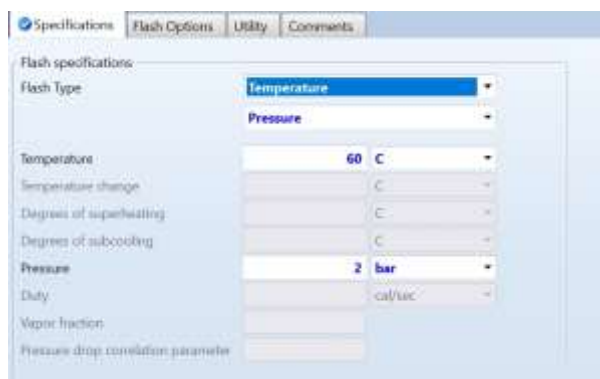
Figure 3.31: Pre-distillation heater for product stream.
