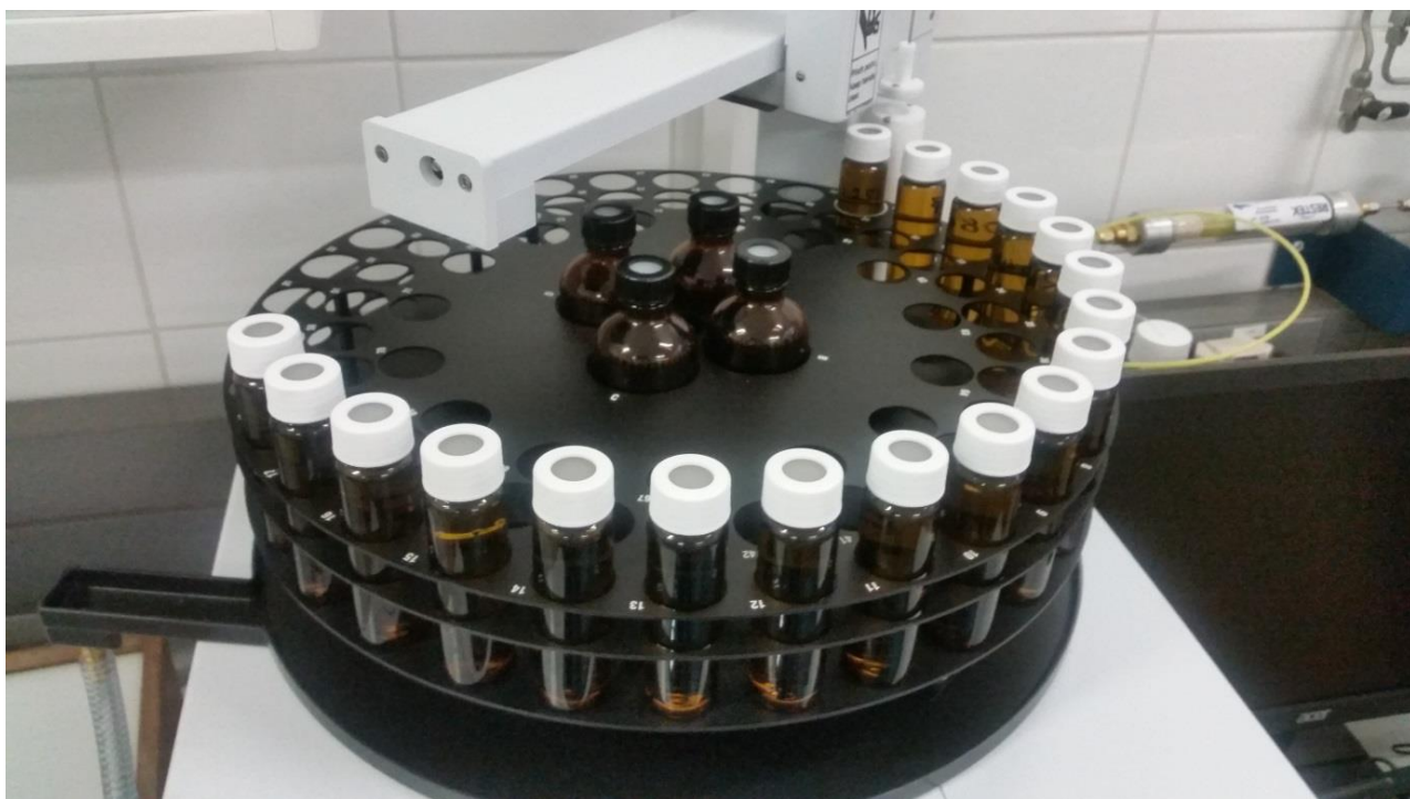
A 3: Teledyne Tekmar Total Carbon Analyser Torch with DOC and BDOC Samples
