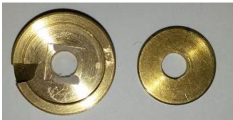
Figure 3.7: An image of EJ 200 scintillator after the cutting and polishing process and being mounted onto the sample holder.
