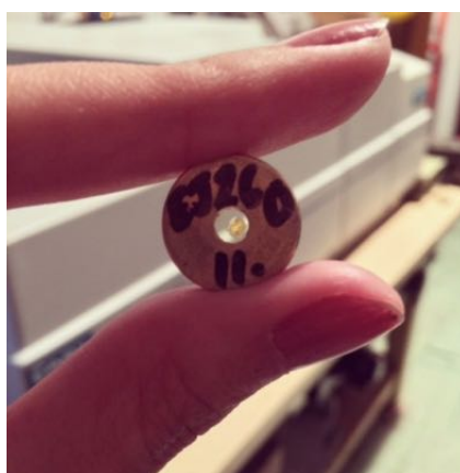
Figure 3.9: An image of EJ 260 after irradiation using a high dose.
