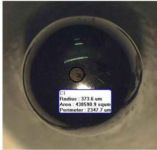
Figure 3. 6 Measurement of the worn area on a 100Cr steel ball.
