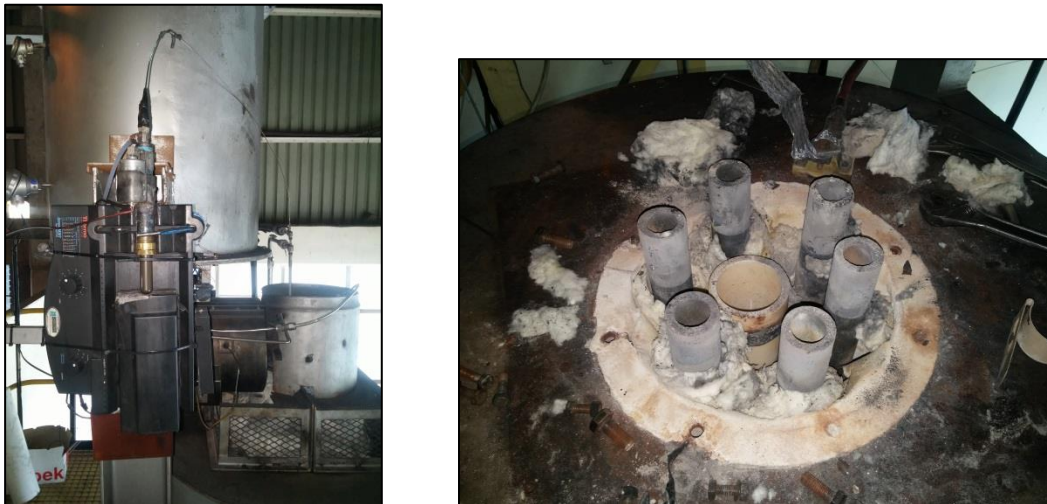
Figure 4-3: (Left) - Mechanical feeder. (Right) - Alumina tube together with the six surrounding heating elements
