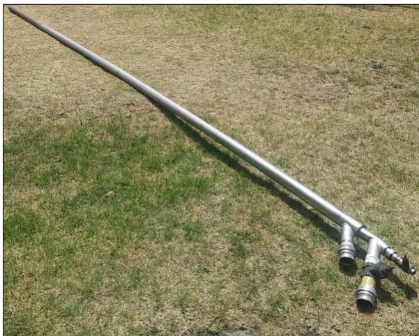
Figure 3-2: Actual water cooled suction pyrometer used
