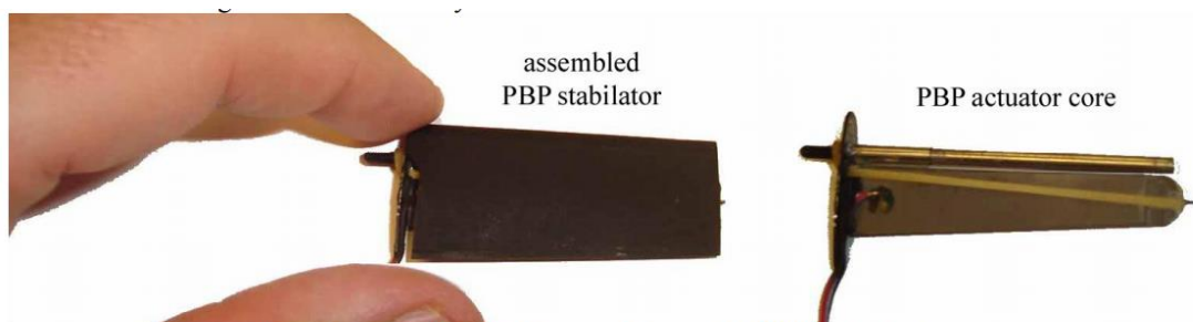
Figure 10 Assembled Stabilator and Assembled PBP Actuator Core
