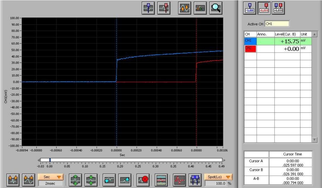
Figure F.4: Time delta measurement using the DAQ
