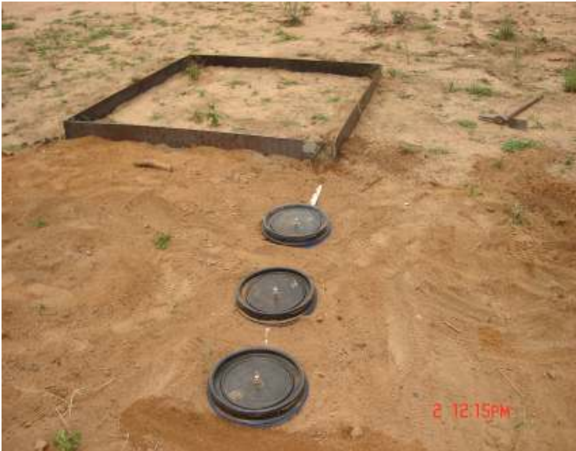
Figure 3.2: Modified runoff collection system
