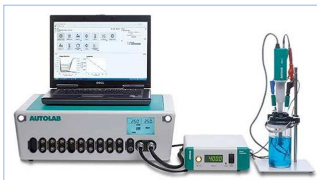
Fig.3.19 (a): Potentiostat set-up (PGSTAT208N, Autolab, Metrohm)
