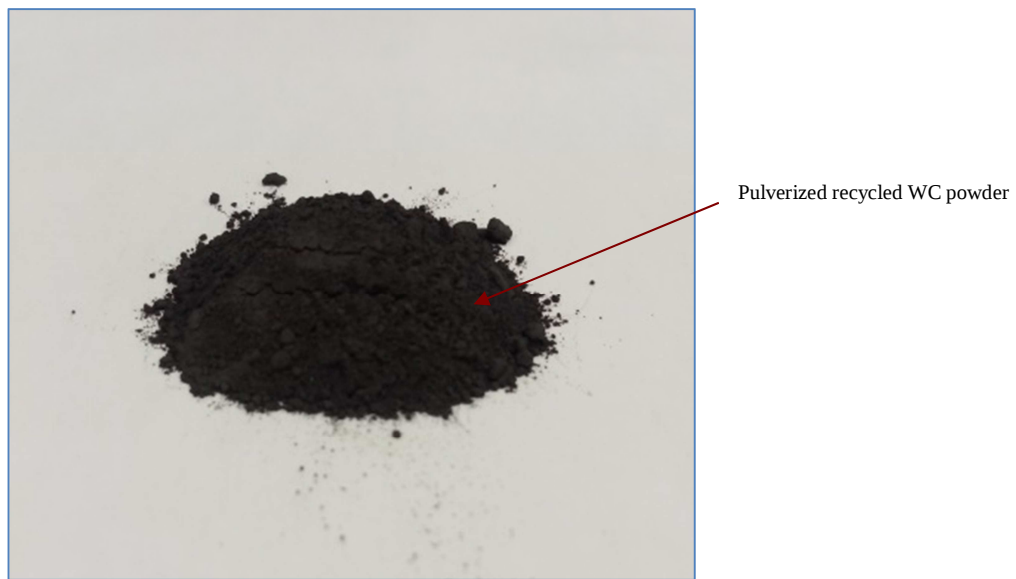
Fig.8.2: Recycled WC powder recovered from cemented tungsten carbide button inserts
