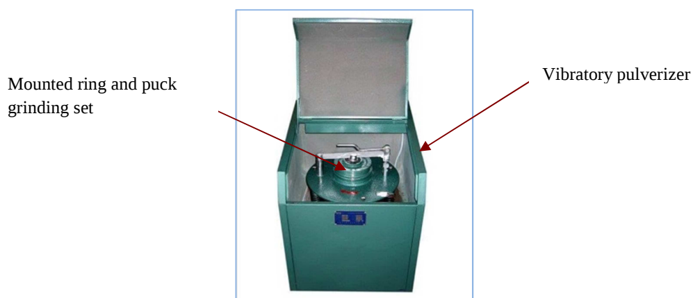
Fig.3.16: Laboratory pulverizer Model 1MZ-100, JXSC, Jiangxi, China
