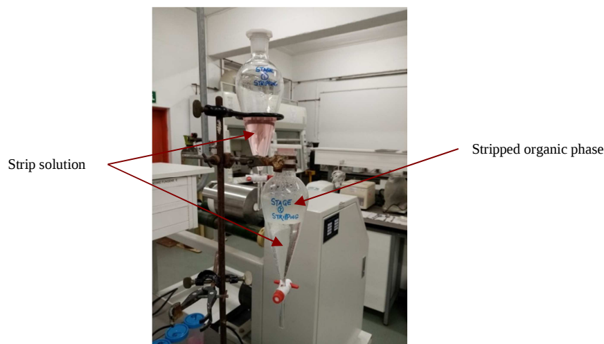
Fig.8.7: Stripping of Co using sulphuric acid
