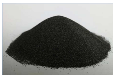
Fig.3.8: Cast tungsten carbide powder
