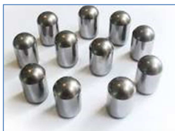
Fig.3.7: Production scrap cemented carbide buttons
