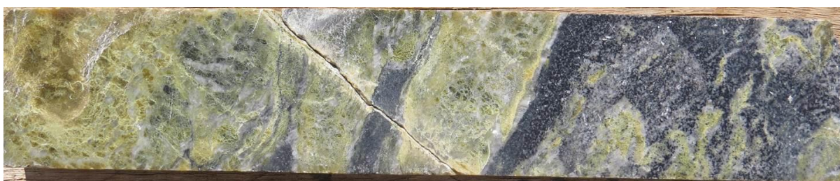
(c) Varied textured dolomite with interbedded chert in drill hole ATS129, at a depth of 185.60 m (25 cm sample, NQ core size)
