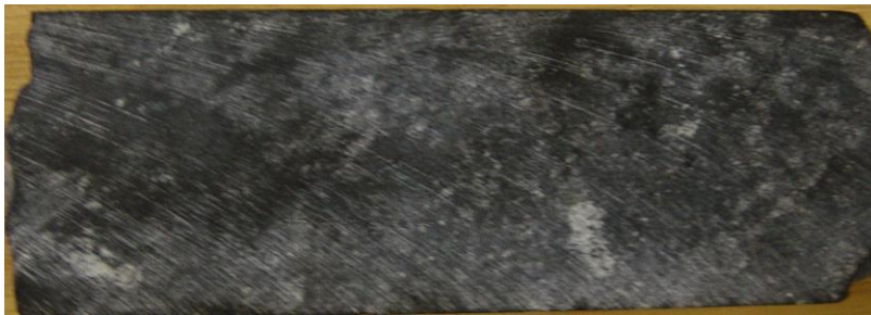
(a) Fine-grained serpentinite in drill hole ITS011, at a depth of 132.05 m (14 cm sample, NQ core size). Original texture of minerals is completely destroyed by alteration
