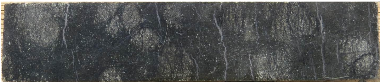
(c) A magnetite-bearing harzburgite with oikocrysts of orthopyroxene in UMT333, at a depth of 1303.15 m (22.5 cm sample, NQ core size). Magnetite occurs in the form of veinlets
