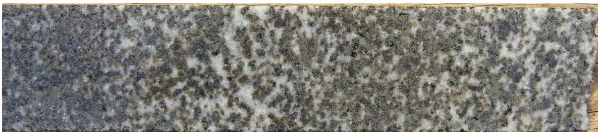
(a) Fine- to medium-grained norite with variable amounts of plagioclase in drill hole UMT063, at a depth of 811.68 m (19 cm sample, BQ core size)
