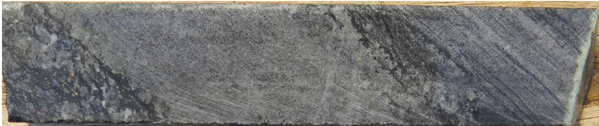
(b) Fine-grained para-pyroxenite showing assimilated sediments in an olivine rich magma in drill hole UMT158, at a depth of 738.22 m (24 cm sample, NQ core size). A zone of olivine (serpentinised) and plagioclase on the left hand side of the diagram represents a magmatic harzburgite. Preserved sedimentary layering is shown on the right hand side of the diagram
