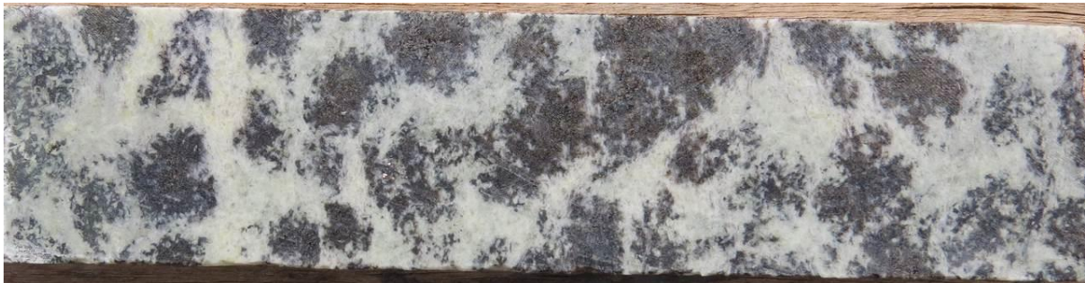
(b) Poikilitic inequigranular mottled anorthosite in drill hole UMT335D1, at a depth of 1464.30 m (25 cm sample, NQ core size)
