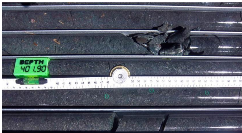
Figure 2.16. Fine- to medium-grained gabbro of the Upper Zone from the Waterberg Project (Platreef workshop 2012)
