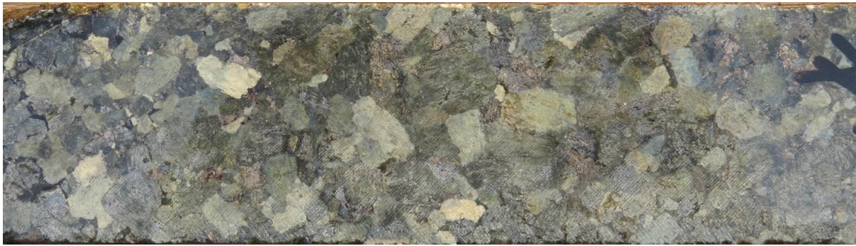
(d) Very coarse-grained olivine, biotite, pegmatoidal orthopyroxenite in drill hole UMT312D1, at a depth of 772.75 m (25 cm sample, NQ core size)
