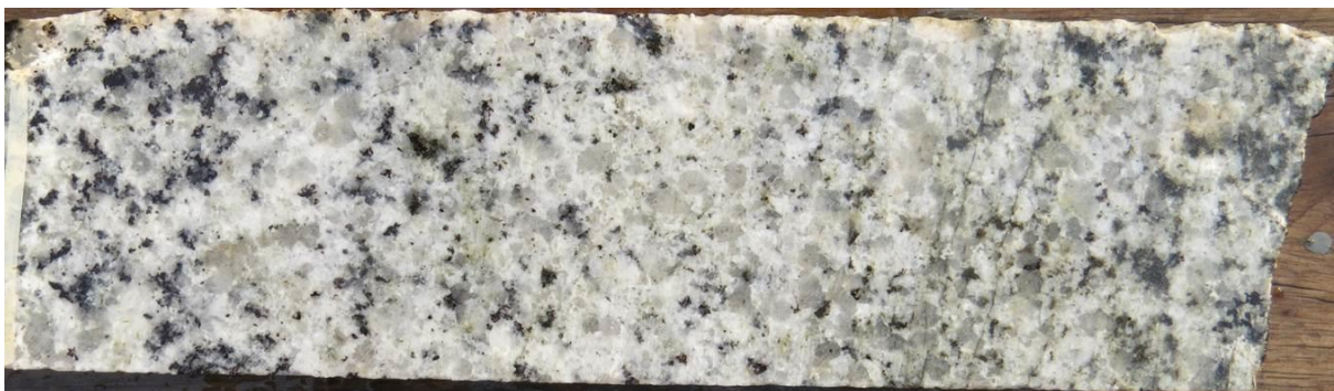
(a) Medium-grained granite vein with pyroxenes and biotite forming a spotted texture in drill hole UMT239, at a depth of 859.31 m (17 cm sample, NQ core size)
