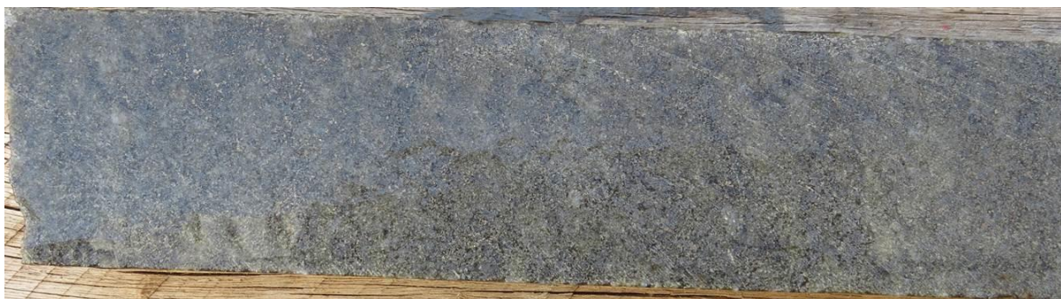
(c) Fine-grained norite with fine-grained sulphides in drill hole UMT060, at a depth of 1198.43 m (20 cm sample, BQ core size). Base metal sulphides are mainly pyrrhotite and pentlandite
