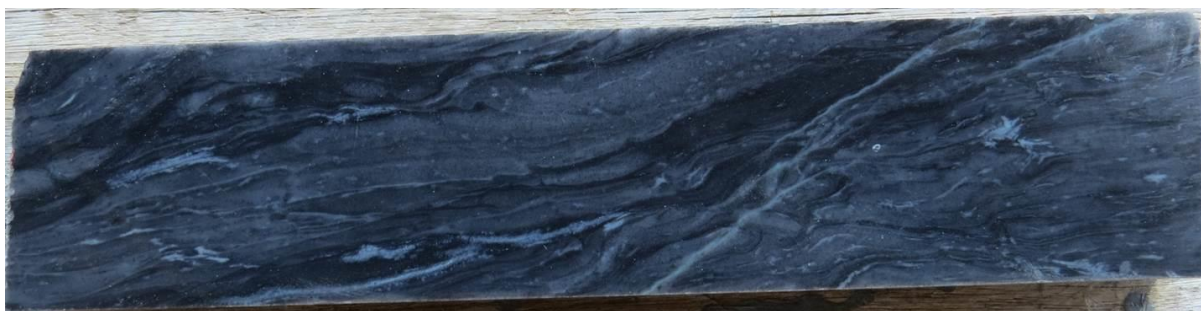
(b) Hornfels displaying porphyroblasts of cordierite-andalusite-pyroxene in a very fine grained groundmass of cordierite-spinel-plagioclase in drill hole ITS097, at a depth of 515.50 m (25 cm sample, NQ core size)
