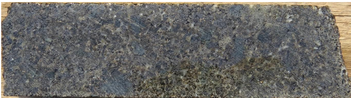
(b) Medium- to coarse-grained feldspathic orthopyroxenite in drill hole UMT064, at a depth of 833.38 m (17 cm sample, BQ core size)
