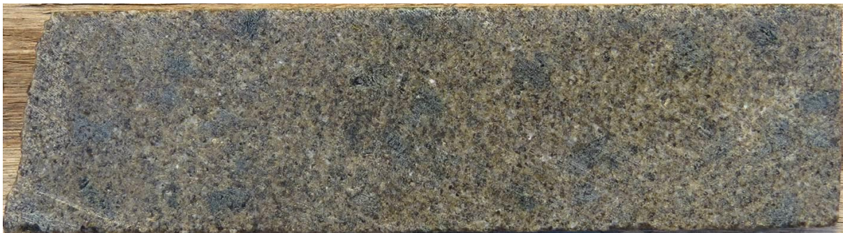
(a) Fine-grained clinopyroxene dominant, porphyritic pyroxenite in drill hole UMT063, at a depth of 817.15 m (17.5 cm sample, BQ core size)
