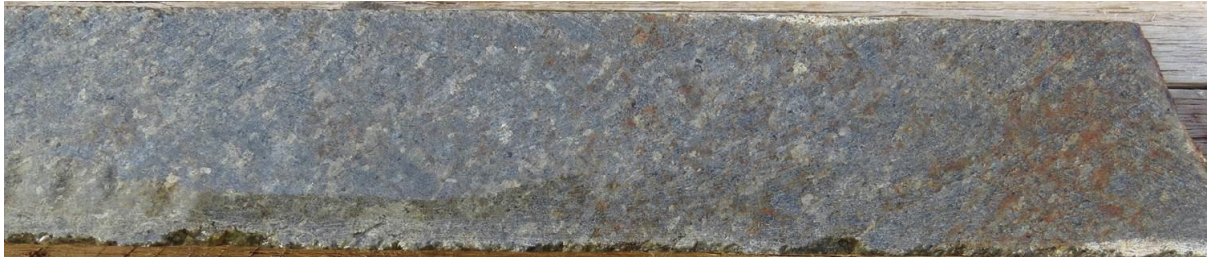
(a) Pyroxenite with elongated orthopyroxene showing fabric in drill hole UMT006, at a depth of 1599.17 m (31 cm sample, BQ core size). Oxidised pyrrhotite and pentlandite shown by orange-brown colour
