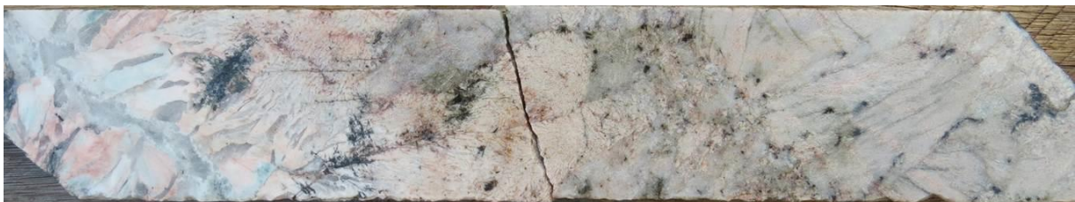
(b) Graphic-textured granite vein with orthoclase and quartz in drill hole UMT158, at a depth of 403.35 m (27 cm sample, NQ core size). Magnetite inclusions are shown by dark spots
