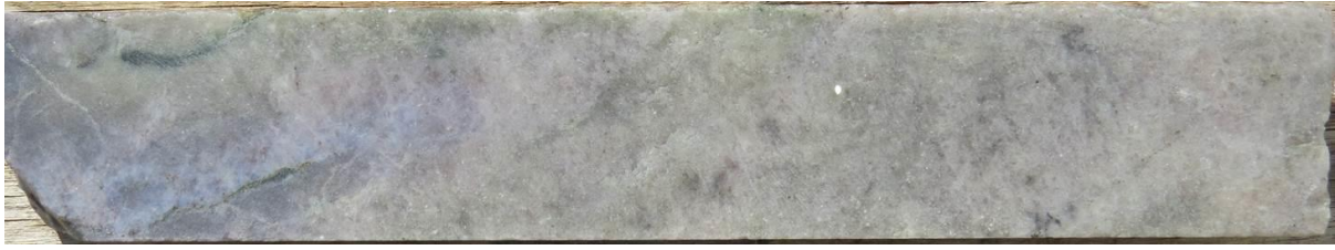
Figure 2.12. Granofels core with chlorite alteration in drill hole UMT088, at a depth of 1509.57 m (28 cm sample, BQ core size)
