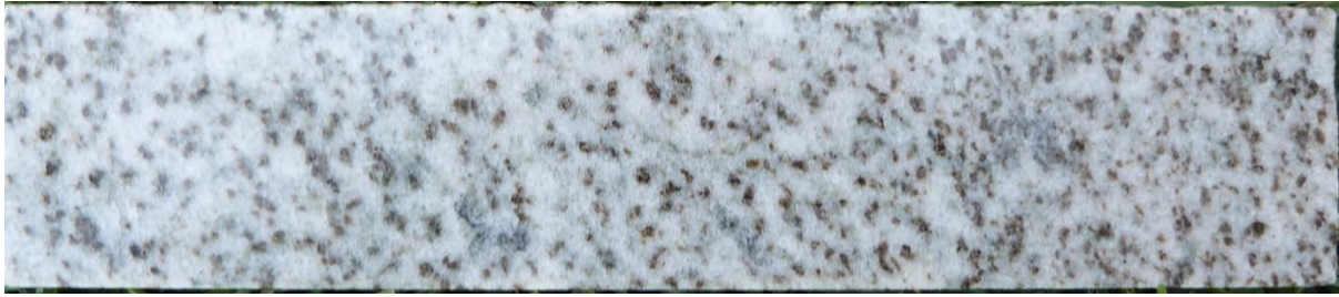
(a) Fine- to medium-grained spotted anorthosite with sub-rounded cumulus orthopyroxenes in drill hole UMT336, at a depth of 1156.20 m (25 cm sample, NQ core size)
