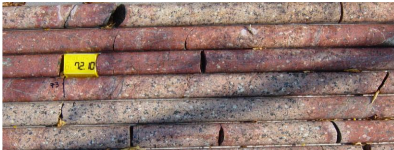
(a) A basement granite core showing variation in potassium content within the basement (NQ core size)
