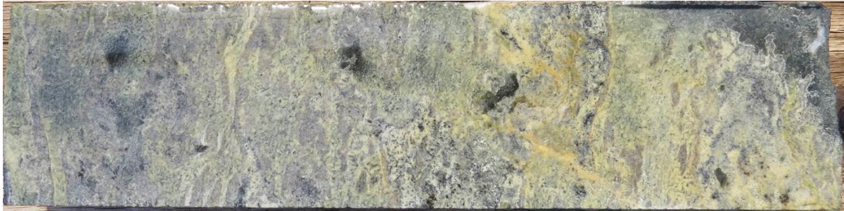
(a) Fine grained calc-silicate (metamorphosed dolomite) in drill hole UMT158, at a depth of 521.62 m (19 cm sample, NQ core size)
