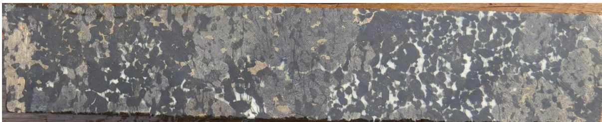
(b) Medium- to coarse-grained feldspathic serpentinised harzburgite with orthopyroxene oikocrysts in drill hole UMT239, at a depth of 807.27 m (25 cm sample, NQ core size). Base metal sulphides occur in the form of interstitial pyrrhotite, pentlandite and chalcopyrite
