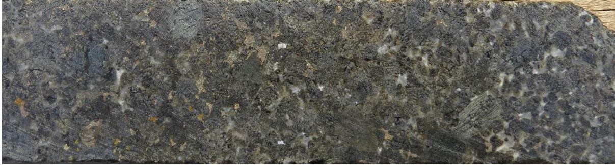
Figure 3.19. T1m sulphide mineralisation showing interstitial blebs of pyrrhotite and pentlandite. Sample length is 22 cm
