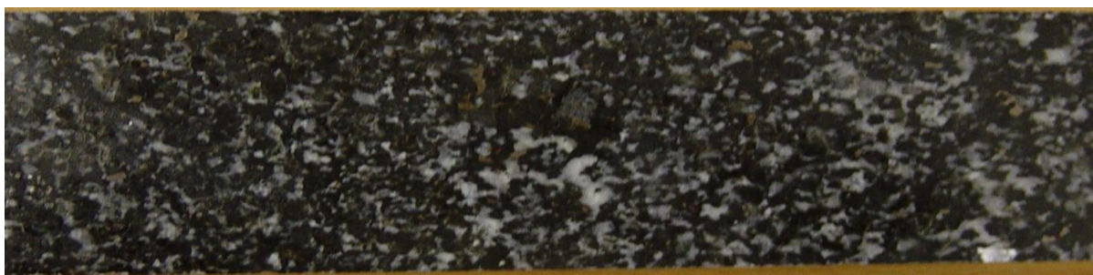
(b) Medium-grained olivine norite with interstitial sulphides in drill hole PA002, at a depth of 647.35 m (29 cm sample, NQ core size). Base metal sulphides are pyrrhotite, pentlandite and chalcopyrite
