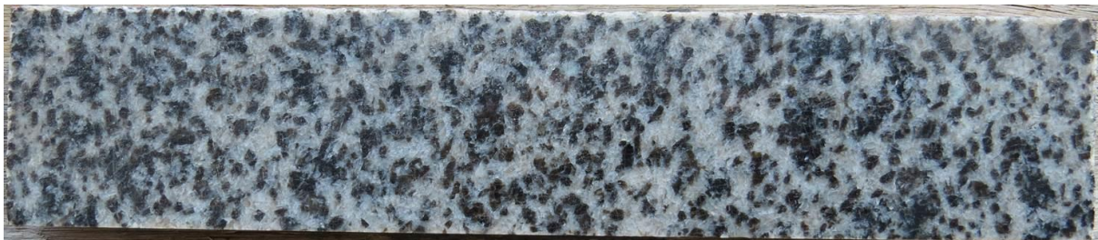
(c) Medium-grained gabbro with rounded cumulus orthopyroxenes in drill hole UMT334, at a depth of 1170.70 m (23.5 cm sample, NQ core size)
