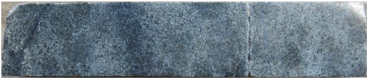
(b) Fine- to medium-grained dunite with > 90 % rounded cumulus olivine in drill hole UMT333, at a depth of 1589.20 m (25 cm sample, NQ core size)
