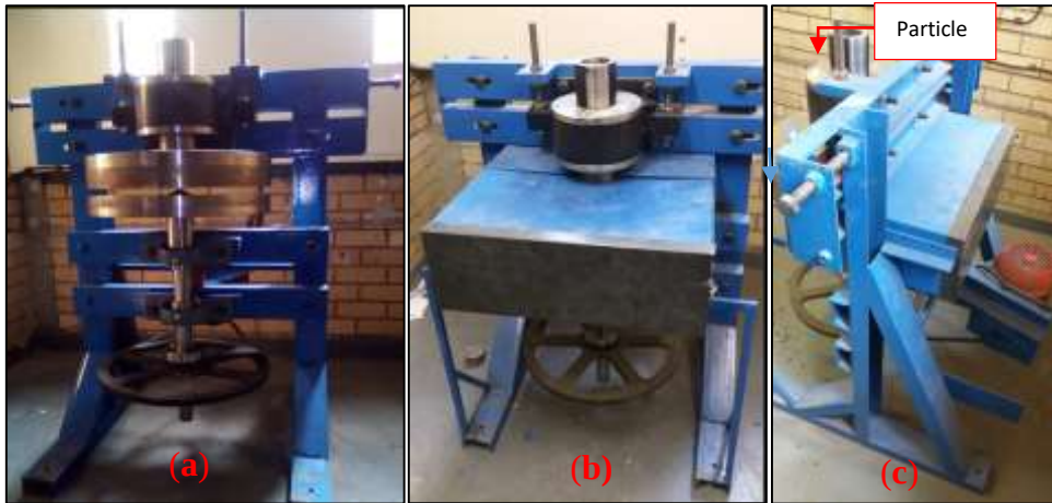
Figure 3. 4: Laboratory prototype of the rotary offset crusher, (a) illustration of the discs (during operation to disc horizontally shifted to the right to provide the offset), (b) Front-end of the crusher fitted with the sample collection box, (c) Back-end of the crusher fitted with the sample collection box.
