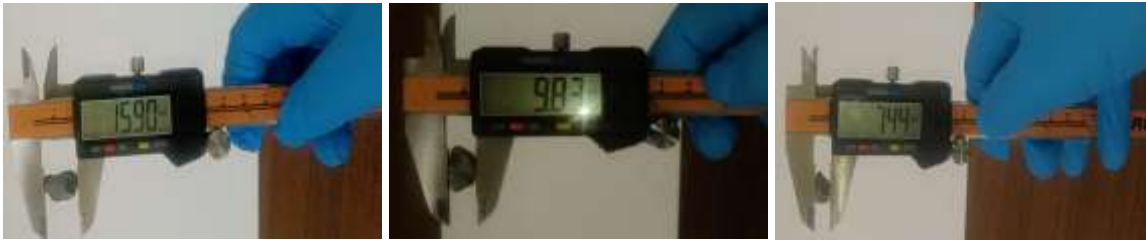
Figure 3. 2: Measurement of length, width and thickness of -9.5+6.7 mm UG2 particle
