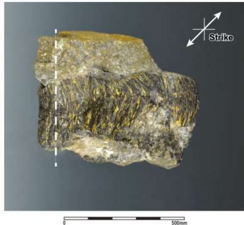
Figure 1. Photograph of CLR sample showing carbon seam bound by a conglomerate footwall and quartzite hanging wall. Photo is taken parallel to strike orthogonal to dip, the white dotted-line shows where the sample was cut
