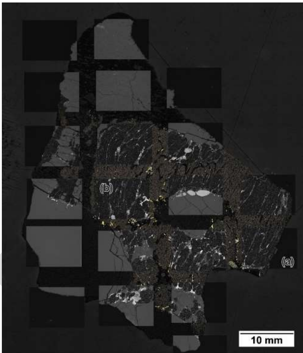
Figure 5 SEM BSE image overlaid over stitched optical microphotograph showing areas mapped by EDS. The BSE overlays highlight materials between the spindles and enhance visibility of uraninite grains, gold and silicate materials, (a) & (b) indicate the positions of Figure 6 (a) & (b) respectively.
