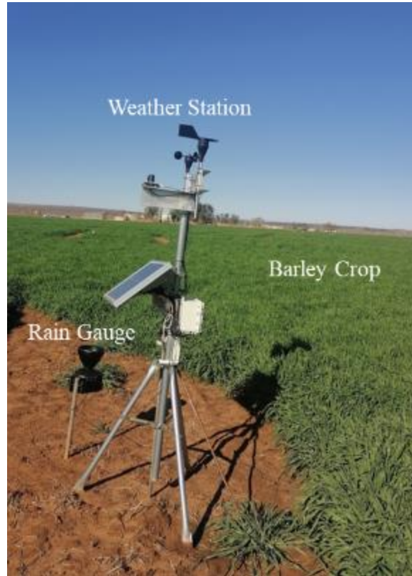
Figure 3.12: Weather station installed north of the lysimeter in the field.
