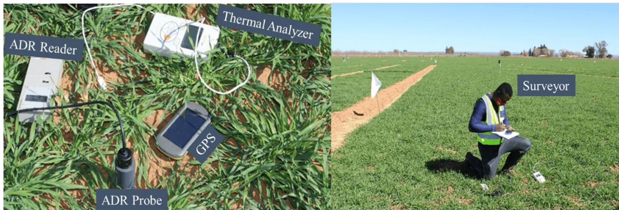
Figure 3.5: Showing the soil water content measuring probe, the thermal analyzer, a GPS and the surveyor during ground measurements.
