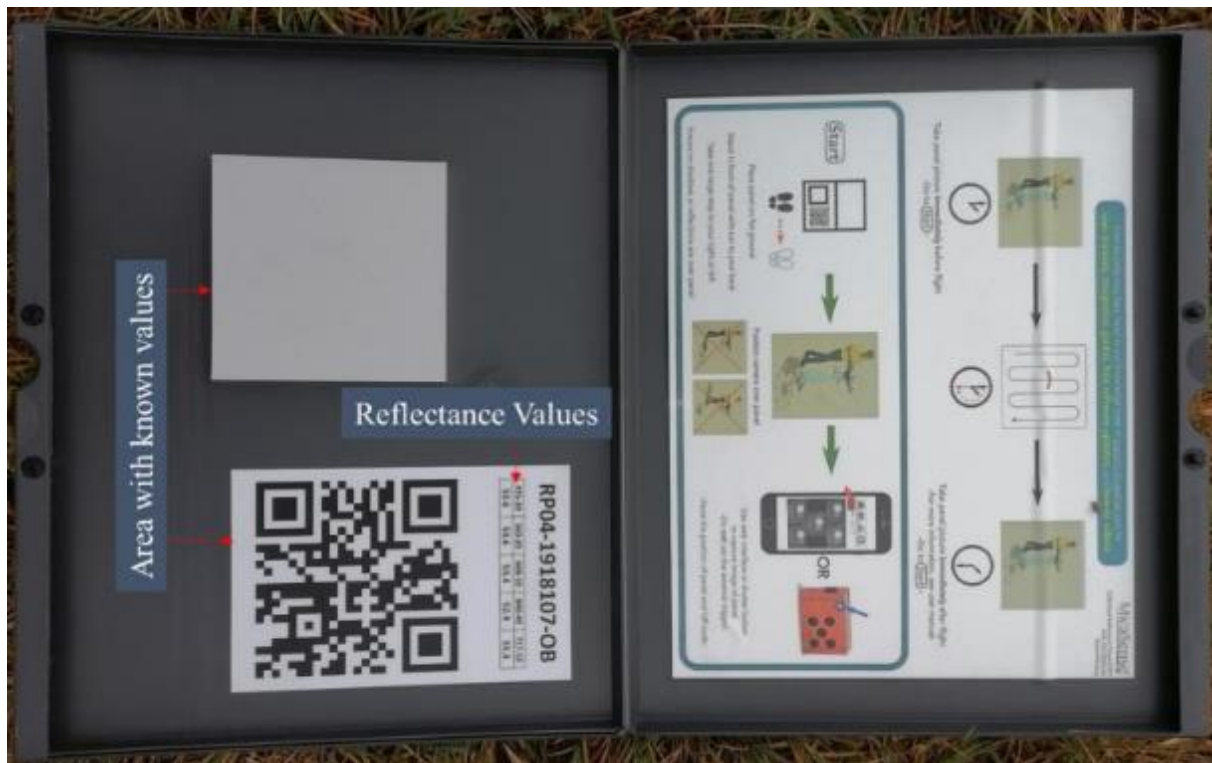
Figure 3.17: Showing the calibration panel for multispectral radiometric calibration.
