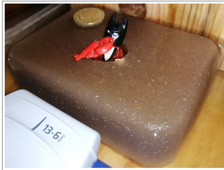
Figure A.7: Additional experimental setup of the probe sonicating a tissue-mimicking phantom with a cylindrical well filled with distilled water. A St Helena £1 coin has been added for scale and three-dimensional perspective.
