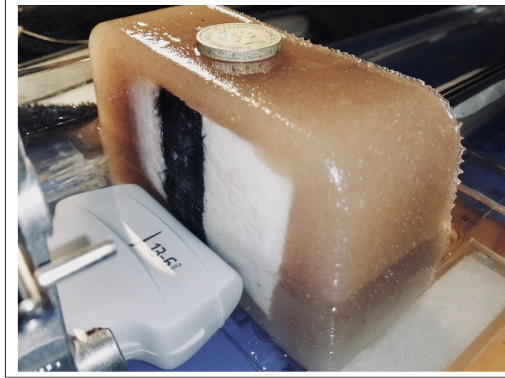
Figure 5.5: Experimental setup of the probe sonicating tattooed pork embedded in a tissue-mimicking phantom. According to practice [140], a St Helena £1 coin with a diameter of 23.44-mm and thickness of 2.80-mm, has been added for scale and for three-dimensional perspective. The dimensions of the phantom were 112 \times 79 \times 40 \text{ mm}^3 .
