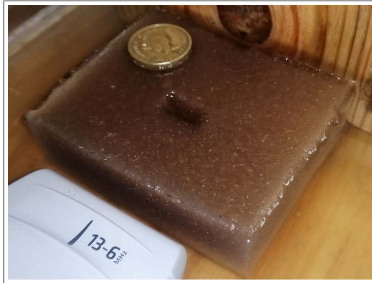
Figure A.5: Experimental setup of the probe sonicating a tissue-mimicking phantom with a cuboid well filled with distilled water. A St Helena £1 coin has been added for scale and three-dimensional perspective.
