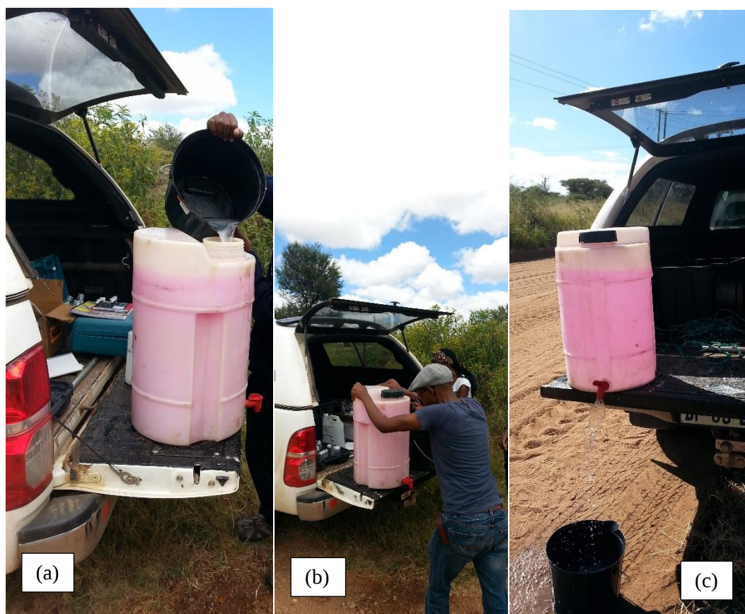
Figure 5.6: Sampling procedure for ^{14}\text{C} and \delta^{13}\text{C} using the drum method.
